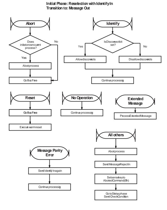
Figure D-13 Message processing after CTS reselects initiator with Identify message
