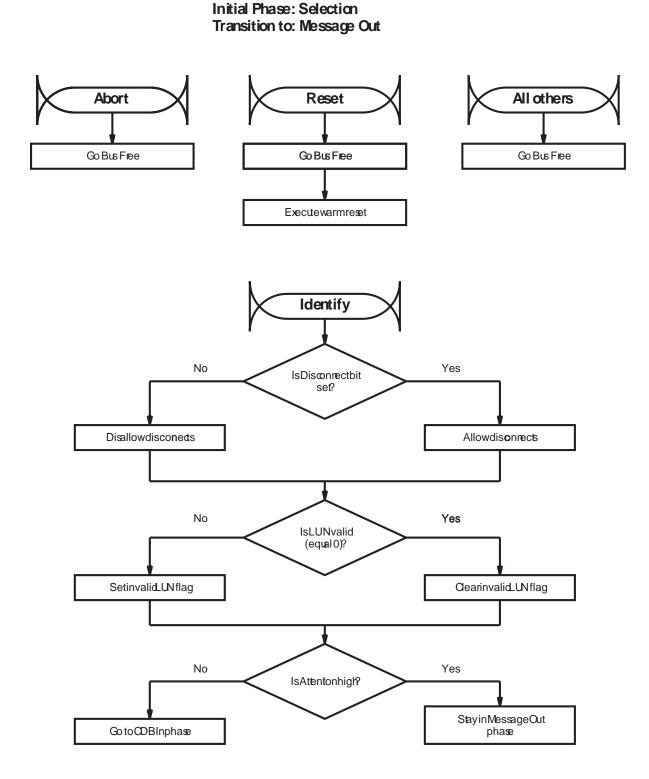
Figure D-1 Message processing after the Selection phase
