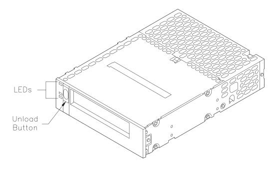
Figure 1-4 Front panel of the EXB-8505
