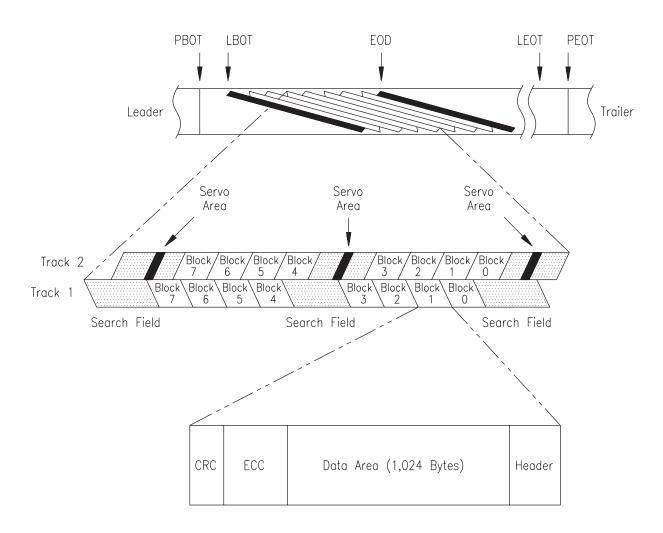
Figure 1-3 Structure of data on tape (8500/8500c physical format)
