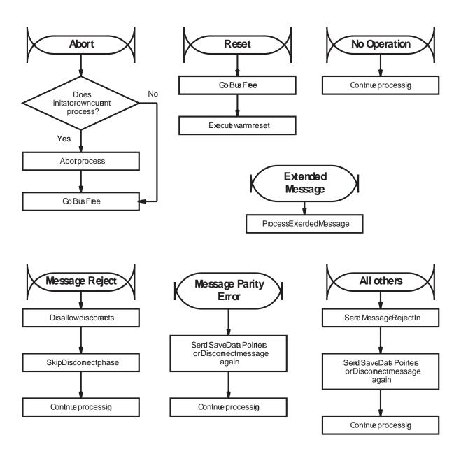
Figure D-14 Message processing while CTS is executing the Disconnect sequence
