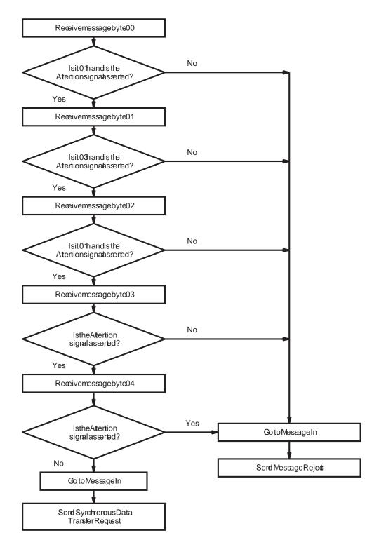
Figure D-5 Message processing of Extended Message Out bytes
