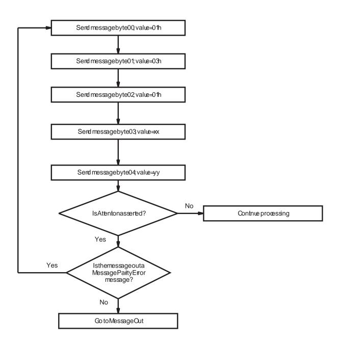
Figure D-6 Message processing for Synchronous Data Transfer Request message
