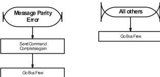
Figure D-12 Message processing during Command Complete Message In phase
