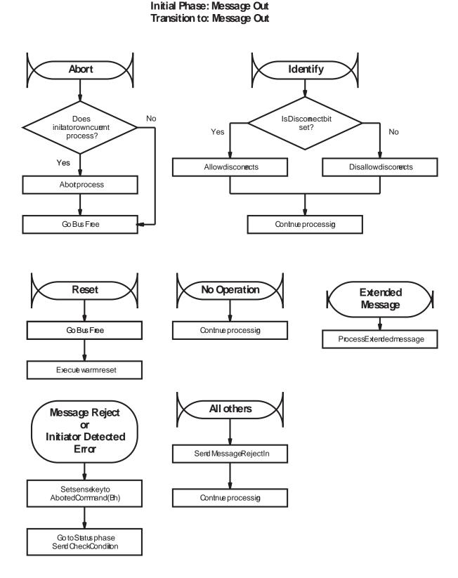
Figure D-4 Message processing after the Command phase and before the Data In phase
