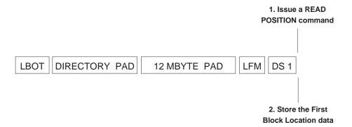
7. Write the READ POSITION data obtained for the various files and blocks in the first data set (DS 1) to the first data set's directory (DIR 1).
