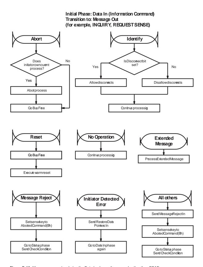
Figure D-10 Message processing during the Data In phase of commands other than READ
