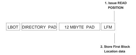
Write the first data set (DS 1) to the tape. While the data set is being written, issue additional READ POSITION commands as desired to obtain the locations of individual files, blocks, and so on contained in the data set.
