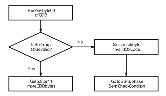
Figure D-3 Processing of CDB bytes
