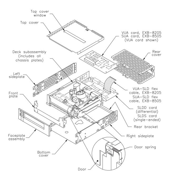
Figure 2-1 Field replaceable units for the EXB-8205 and EXB-8505
