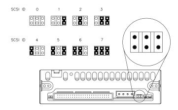
**Note:** If you are using a remote switch to set the SCSI ID, remove the jumpers from the jumper block and attach the switch connector. Make sure that the switch is no more than 30.5 cm (12 inches) from the jumper block.
