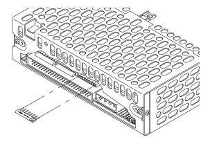
If the tape drive uses R-packs: Make sure the R-packs are installed if the tape drive is at the end of the SCSI bus. If you need to install R-packs, make sure that pin 1 of each R-pack is aligned with pin 1 of the socket and that no pins are bent. If the tape drive is not at the end of the SCSI bus, use a pair of flat-nose pliers to carefully grasp each R-pack at the center and pull it straight out.
