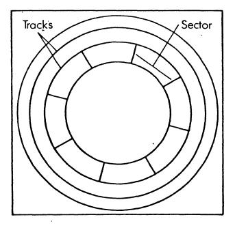
When a disk is formatted, the system organizes it into a series of coded sectors. When you clear a disk, all data is erased, but not the codes and sectors.
