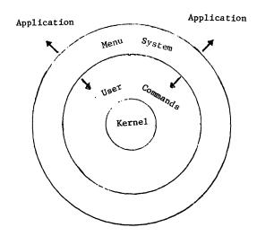
Use the terminal and keyboard to communicate with the operating system's three parts: the kernel, the user commands, and the menu system.
