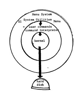
When you select a command from a menu, the menu system tells the command interpreter to run a user command. The actual processing involved is carried out by the Fortune Operating System kernel.
