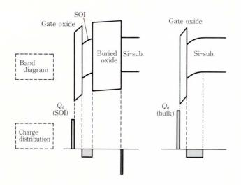
Fig. 7-Band diagram and charge distribution for MOSFET.
