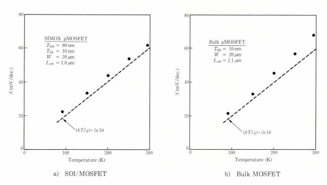
Fig. 8 – Temperature dependence of subthreshold swing.
