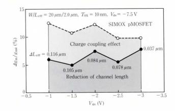
Fig. 12-Effects of trapped electrons in gate and buried oxide on transconductance.
