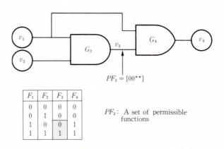
Fig. 1 – An example of permissible functions.
