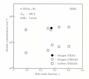
Fig. 3 – The variation of oxygen and carbon concentration in n-AlGaAs with the AlAs mole fraction.
