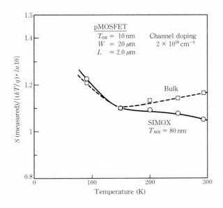
Fig. 9-Temperature dependence of normalized subthreshold swing.
