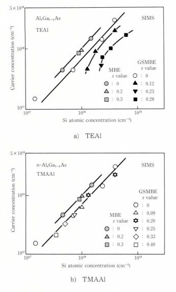
Fig. 6-The dependence of the carrier concentration of n-AlGaAs (x = 0.0.4) on the Si atomic concentration using TEAl and TMAAl.
