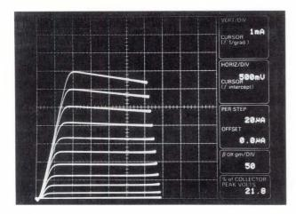
Fig. 10-Common-emitter I - V characteristics of the HBT. The vartical scale is 1 mA/division and the horizontal scale is 500 mV/division. The base current is 20  $\mu$  A/step.
