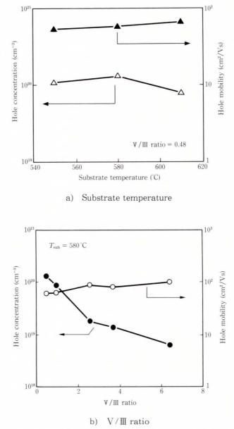
Fig. 7 – The variation of GaAs hole concentration with substrate temperature and V/III ratio.
