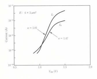
Fig. 11-Gummel plots for a carbon doped base HBT.
