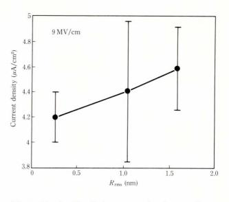
Fig. 6 – Fowler-Nordheim current for three surface roughnesses.
