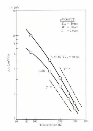
Fig. 6 – Temperature dependence of field effect mobility.
