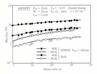
Fig. 10-Change in transconductance versus stress time.
