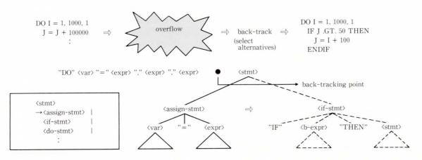
Fig. 3 – An example of back-tracking caused by a loop.
