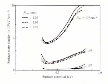
Fig. 8-Surface state density for three surface roughnesses when constant current is injected.
