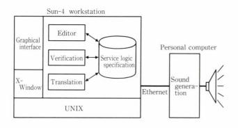
Fig. 6-Configuration of prototype system.
