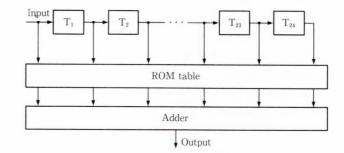
Fig. 6-Digital transversal filter.
