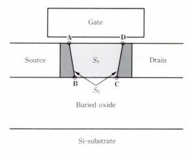
Assumptions for points **A**, **B**, **C**, and **D**: a) Lateral electric field is zero. b)  $E_t = E_t$ .
