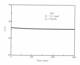
Fig. 12–Variation of gain  $(I_c/I_b)$  with electrical stress time.
