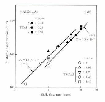
Fig. 5 – The variation in Si atomic concentration with the Si<sub>2</sub>H<sub>6</sub> flow rate for n-AlGaAs using TEAl and TMAAl.
