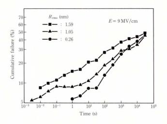
Fig. 7 – Time-dependent dielectric breakdown characteristics for three surface roughnesses.
