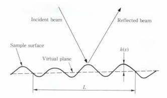
Fig. 2 – Measurement of the surface roughness with an optical interferometer.
