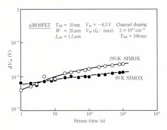
Fig. 11-Change in threshold voltage versus stress time.
