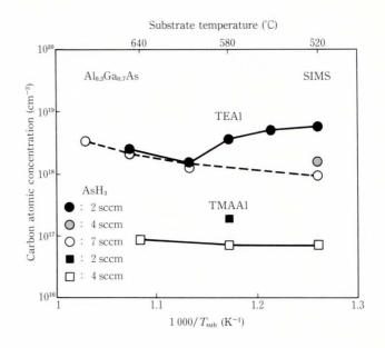
Fig. 1- The variation of the background carbon concentration with  $T_{\rm sub}$  and  ${\rm AsH_3}$  flow rate for undoped AlGaAs grown using TEAl and TMAAl.
