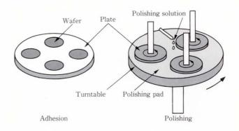
Fig. 1 – Wafer polishing system. The wafers are attached to the rotating plate and the polishing pads to the rotating turntable. T. Nakanishi et al.: Influence of Silicon Surface Roughness on Time-Dependent Dielectric Breakdown
