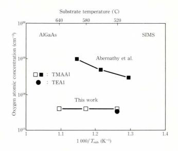
Fig. 2-The dependence of the oxygen concentration on  $T_{sub}$  for undoped AlGaAs. Abernathy et al. reported for AlGaAs grown by using the same combination of source gases (TMAAl, TEGa and AsH<sub>3</sub>)<sup>19)</sup>.
