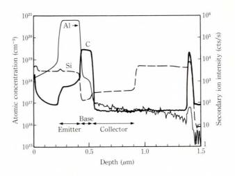
Fig. 9-SIMS depth profile for a HBT structure.
