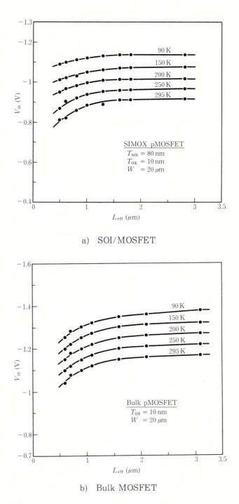
Fig. 2–Threshold voltage versus  $L_{\rm eff}$  for various temperatures.
