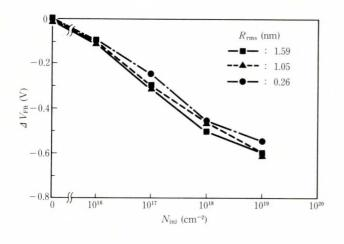
Fig. 9 – Flat band voltage shift under constant current stress.
