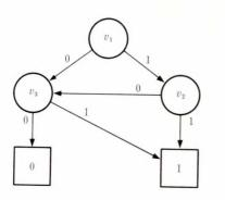
Fig. 2-BDD representation of  $F = v_1 \& v_2 + v_3$ .
