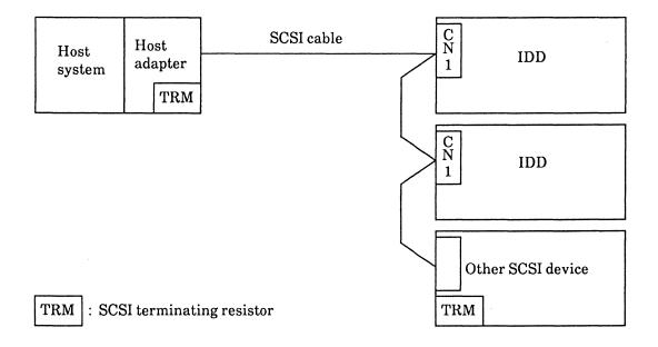
Figure 5.1 SCSI bus connections (1 of 2)
