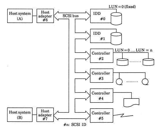
Figure 1.3 System configuration
