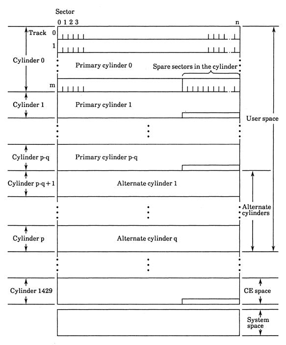
\*1 Spare sectors on the last track in each cylinder are not necessarily placed at the end of the track because of a track skew or a cylinder skew. (Details are explained in Section 3.1.3.)
