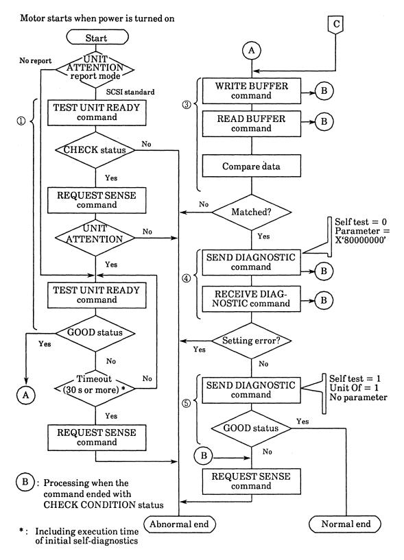
Figure 5.7 Checking the SCSI connection (A)
