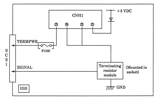
Figure 5.5 Configuration of SCSI terminating resistor circuit
