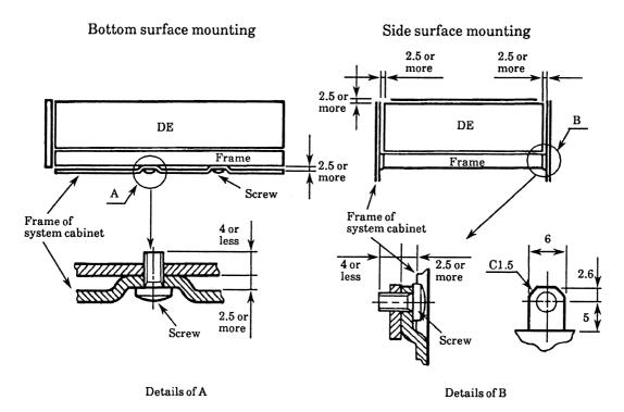
Figure 4.5 Mounting frame structure
