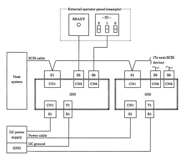
Figure 4.20 Cables connection
