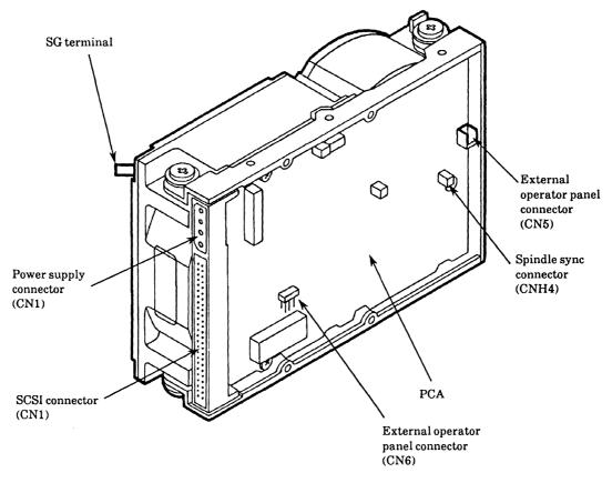
Figure 4.12 Positions of connectors (M2624S)
