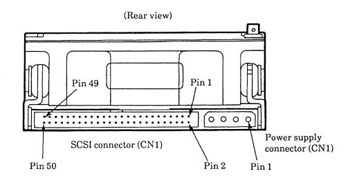
Figure A.1 Positions of connectors, pins, and terminating resistor
