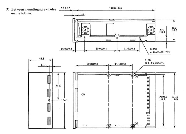
Figure 4.3 Exterior dimensions (M2624S with front panel)
