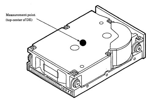
Figure 4.1 DE surface temperature measurement point
