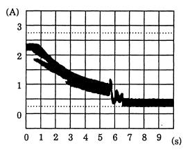
Figure 4.7 Current waveform (+12 VDC)
