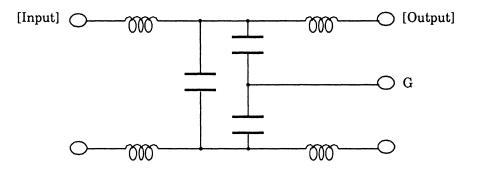
Figure 4.11 AC noise filter (recommended)
