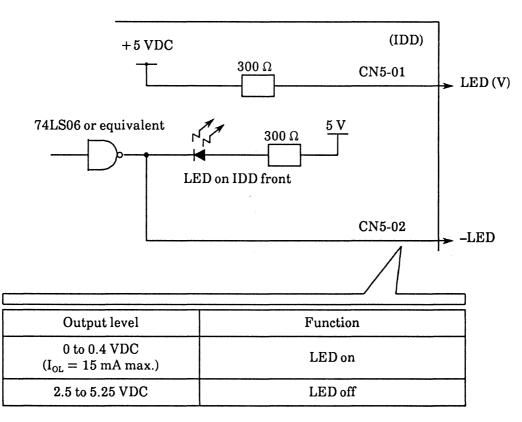
Figure 4.19 Output signal for external LED
