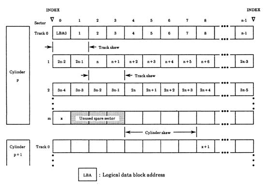
Figure 3.5 Track skew/cylinder skew
