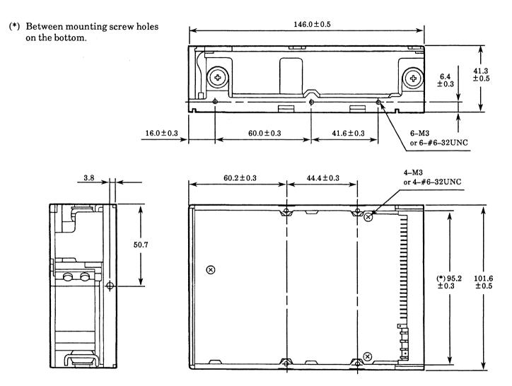
Figure 4.2 Exterior dimensions (M2624S without front panel)
