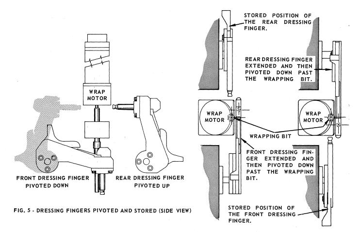
FIG. 6 - DRESSING FINGERS PIVOTED AND STORED (TOP VIEW)
