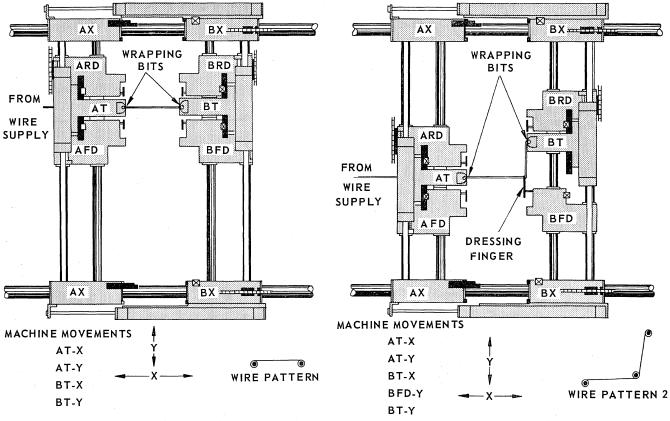
FIG. 8 - FINAL CARRIAGE POSITIONS PATTERN 1
