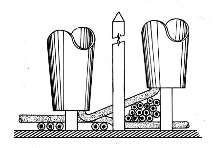
FIG. 16 - CHANNEL BUILD-UP EFFECT ON SHORT Z-1 WRAPS WHEN THEY ARE NOT PUT ON FIRST
