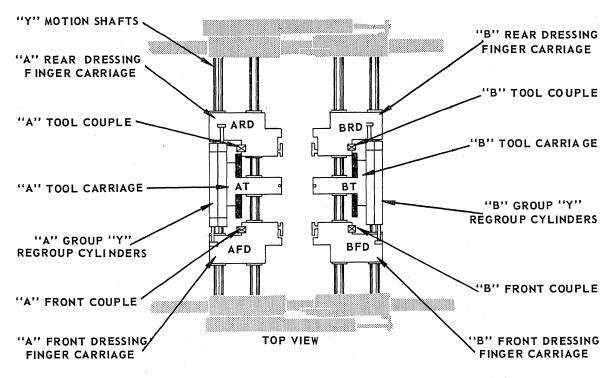
FIG. 2 - "Y" MOTION CARRIAGES AND REGROUP CYLINDERS
