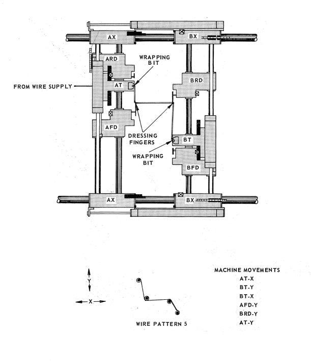
FIG. 12 - FINAL CARRIAGE POSITIONS PATTERN 5
