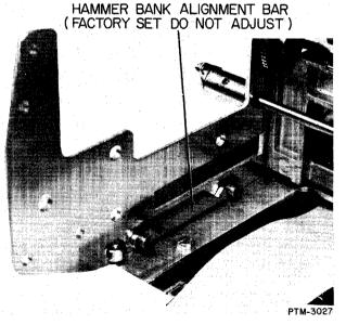
Figure 5-33. Hammer Bank Alignment Bar.
