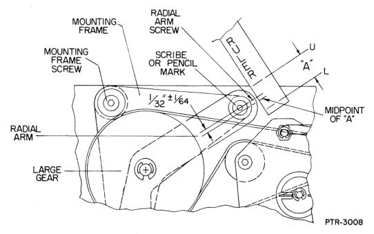
Figure 5-44. VTFF Adjustment Mechanics.
