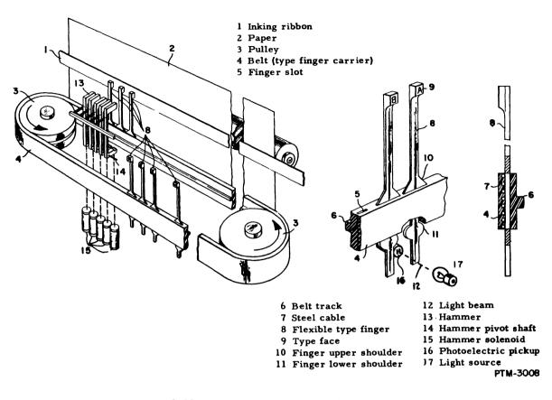
Figure 3-25. Hammer and Print Belt Assembly.
