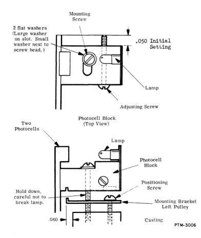
Figure 5-36. Preliminary Photocell Adjustment.
