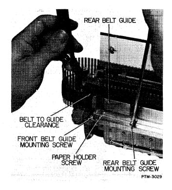
Figure 5-26. Rear Belt Guide Adjustment.
