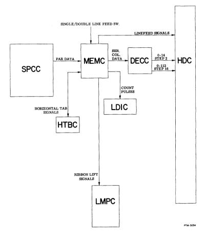
Figure 3-37. Functional Block Diagram of MEMC, DECC, HTBC, and LDIC.
