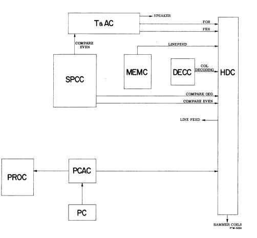
Figure 3-38. Functional Block Diagram of HDC and T&AC
