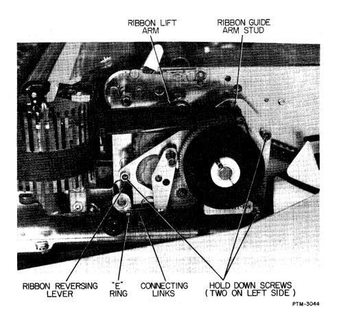
Figure 5-15. Ribbon Reversing Mechanism Hardware.
