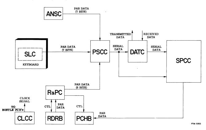
Figure 3-35. Functional Block Diagram of CLCC, SLC, ANSC, R&PC, and PSCC.
