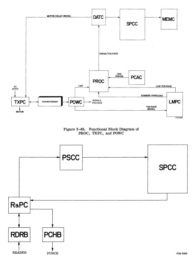
Figure 3-41. Functional Block Diagram of RDRB and PCHB
