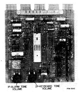
Figure 5-39. T&AC Board Adjustments.
