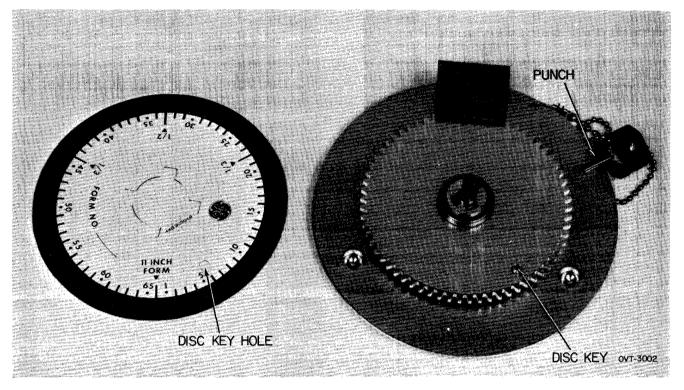
Figure 3-20. Programmable Disc and Disc Punch.
