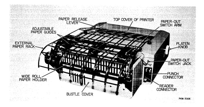
Figure 3-4. Left Rear View of Printer.
