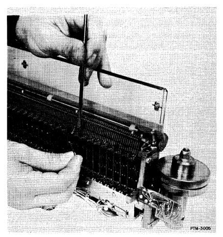
Figure 5-34. Clevis Disconnect.
