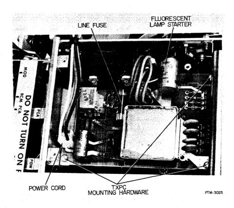
Figure 5-11. TXP Board Mounting.
