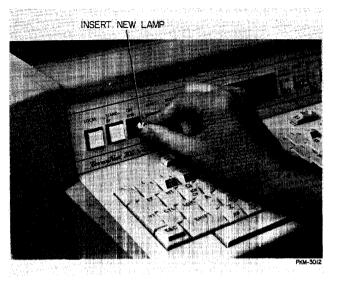
Figure 3-13. Installing Lamp.
