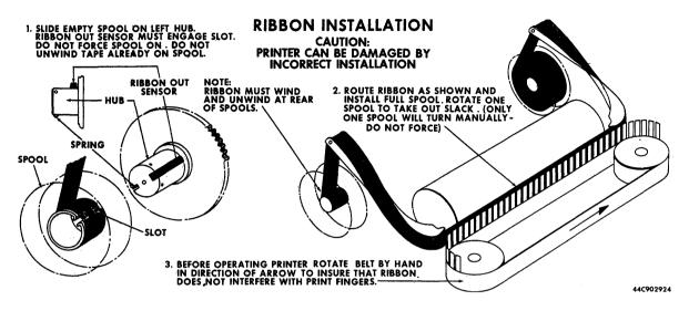
Figure 3-8. Ribbon Installation.
