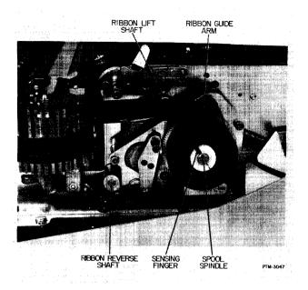
Figure 3-27. Ribbon Spool Drive System. (Right Side View)
