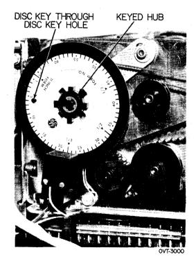
Figure 3-22. Programmed Disc Mounting
