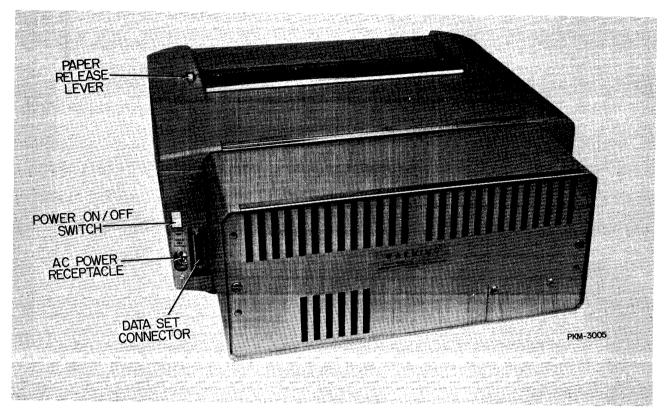
Figure 3-3. Right Rear View of Printer.
