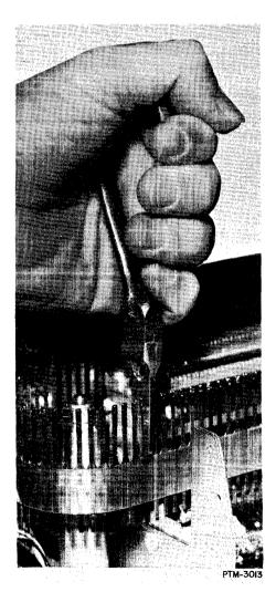
Figure 5-19. Print Finger Removal.
