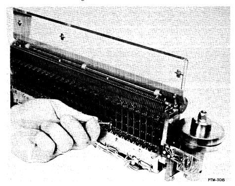
Figure 5-35. Clevis and Plunger Removal.
