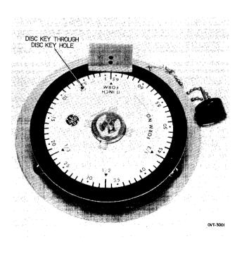
Figure 3-21. Programmable Disc on Disc Punch.
