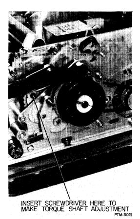
Figure 5-24. Torque Shaft Adjustment.
