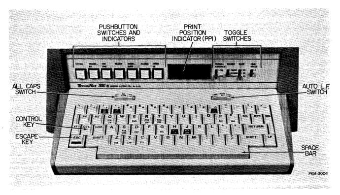
Figure 3-1. KSR Keyboard and Control Panel
