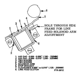
Figure 5-20. Line Feed Solenoid Adjustment.
