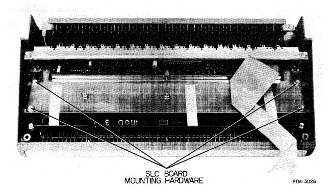
Figure 5-8. Sense Line Combined Board Mounting.
