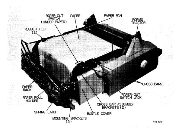
Figure 3-17. External Paper Handler Using Forms Tractor.
