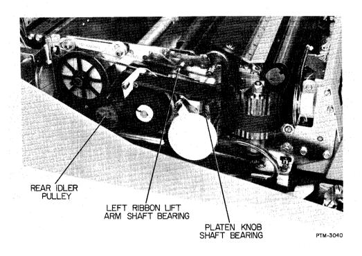
Figure 5-3. Lubrication Points - Printer Left Side.
