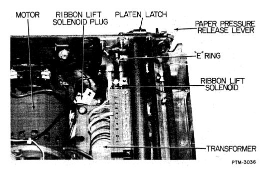
Figure 5-12. Internal Printer Components, Right Side.
