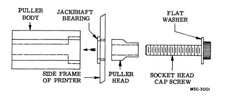
Figure 5-22. Bearing Puller.
