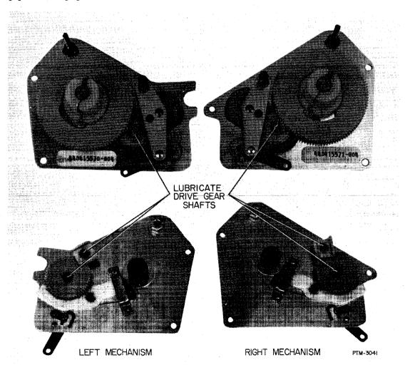
Figure 5-2. Lubrication Points - Ribbon Reversing Mechanisms.
