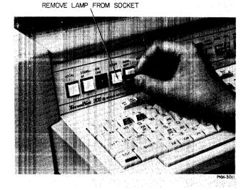
Figure 3-12. Removing Lamp.
