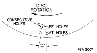
Figure 5-43. VTFF Adjustment Range "A" on Disk.
