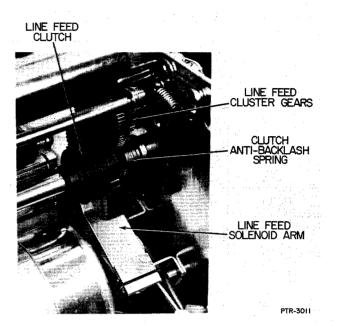
Figure 3-30. Line Feed Mechanics.
