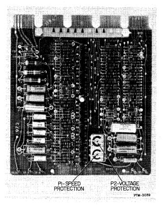
Figure 5-38. PROC Board Adjustments.
