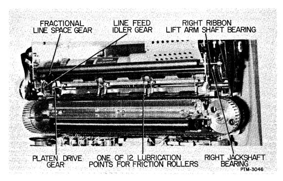
Figure 5-5. Lubrication Points - Printer Interior.
