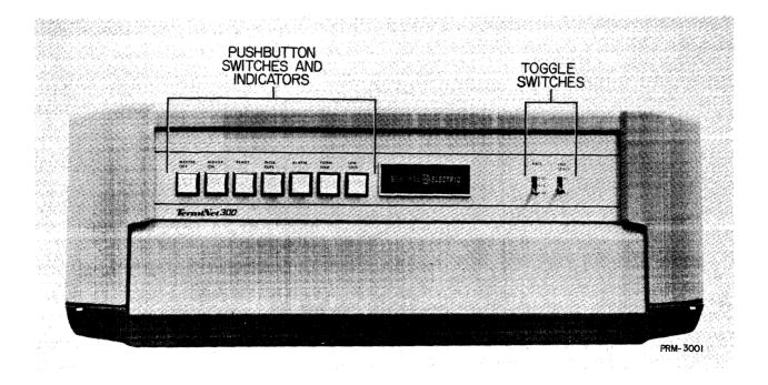
Figure 3-2. RO Control Panel
