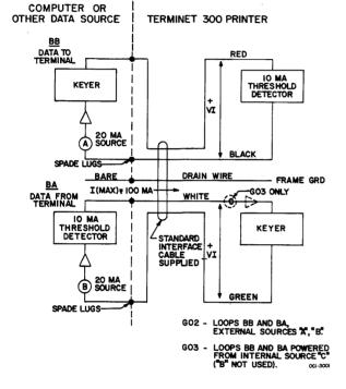
Figure 3-16. Current Loop Interface System.
