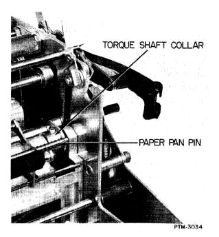
Figure 5-23. Paper Pressure Adjustment.
