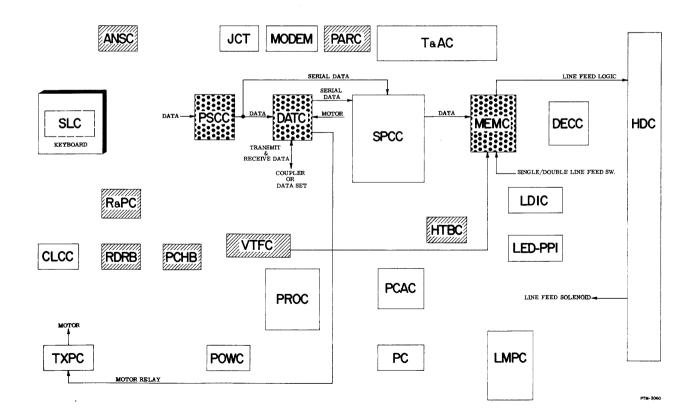
Figure 4-2. Motor and Line Feed Circuits
