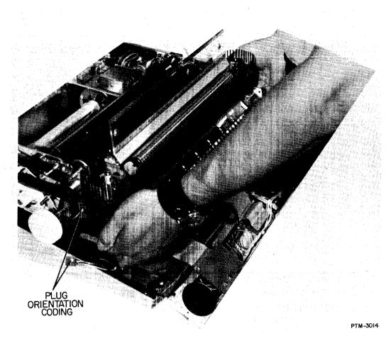
Figure 5-32. Hammer Bank Removal.
