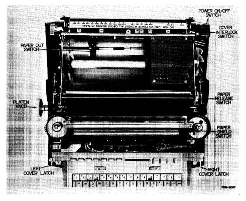
Figure 3-5. Switch Locations and Manual Controls.
