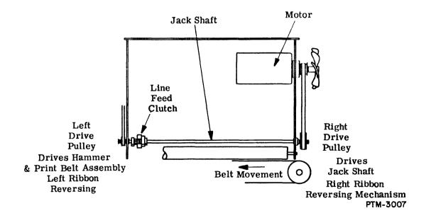
Figure 3-28. Drive Mechanism
