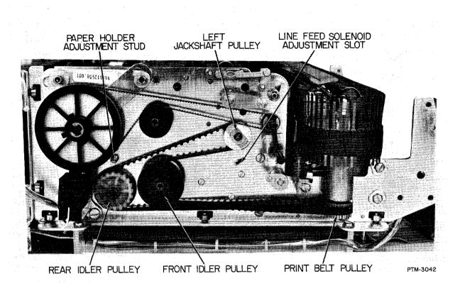
Figure 5-16. Left Drive Belts and Pulleys.
