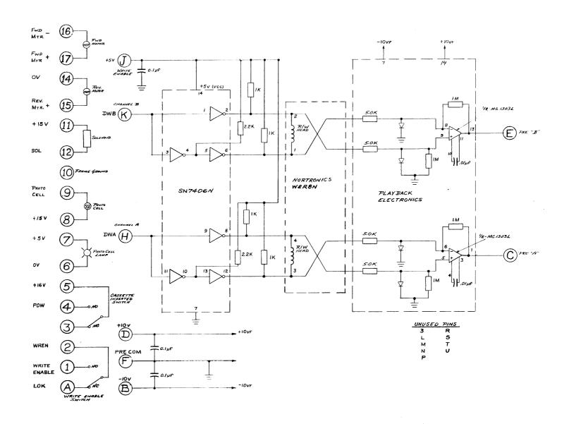
Figure 4-11. TCA Deck/Preamp (44C400175, Rev. 1) - A1, A2, and A3 Models TCA
