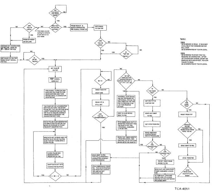
Figure 3-10. Functional Flow Diagram of Read Sequence of Operation
