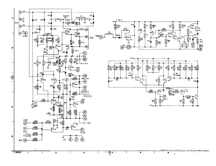
Figure 4-5. TPS/1 Printed Circuit Board (44C420202, Rev. 11) - A1 Model TCA
