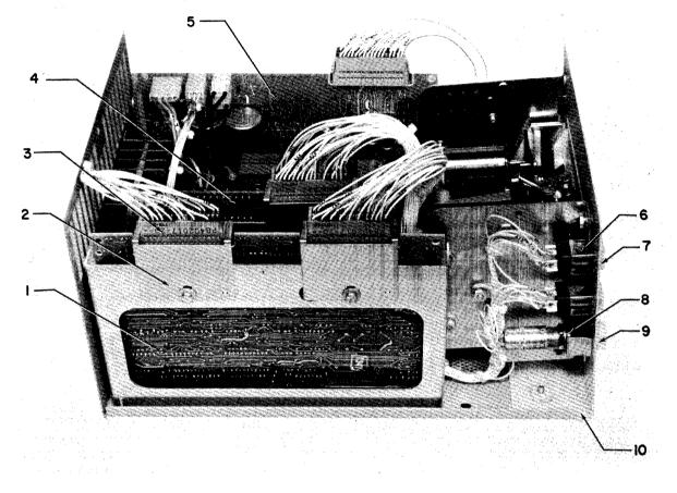
Figure 6-1. Printed Circuit Boards and Connectors and Brackets
