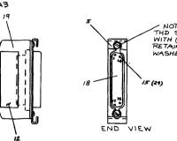
NOTE: USE (2) 4-40 THD SCREWS PACKED WITH (PART 5) LOCK RETAINER, DISCARD LOCK WASHERS AND NUTS.
