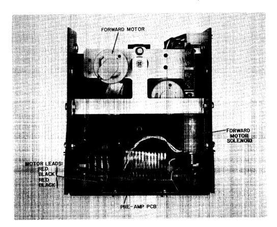
Figure 5-7. Forward Motor Solenoid
