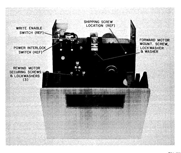
Figure 5-6. Forward Motor Mount Retaining Screw
