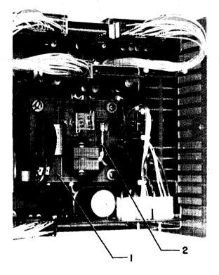
TCA-4040 Figure 6-2. TLP Printed Circuit Board and Fuses
