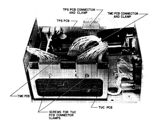
Figure 5-9. PCB Removal
