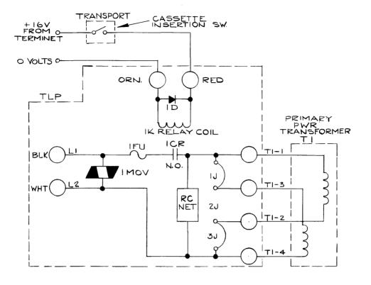
GOI 120 VAC 50/60 HZ IJ, JJ IN ; 2J OUT IFU = I AMP GO2 240 VAC 50/60 HZ 2J IN ; IJ, JJ OUT IFU = 0.5 AMP
