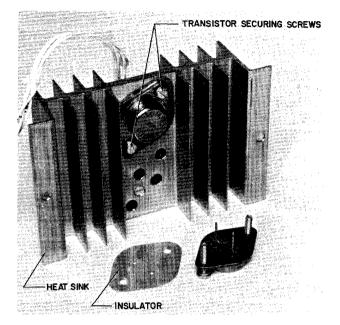
TCA-4037 Figure 5-12. Power Transistor Removal
