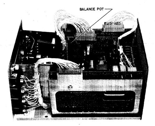
Figure 5-13. Balance Pot on TMC PCB
