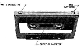
TCA-4030 Figure 3-6. Write Lockout Tab
