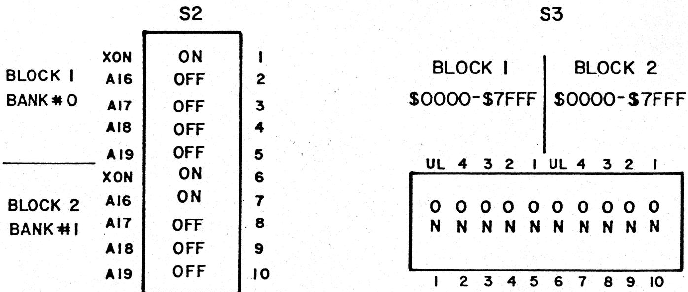
FIG. 4: TWO SEPARATE 32K BANKS \$0000-\$7FFF BANKS 0 & 1
