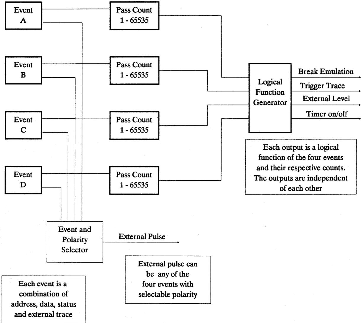
Fig. IV-1 Event and Sequencing Diagram
