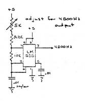
Circuit of 4000 Hz oscillotor; Use this Circuit if a more precise and stable Source of 4000 Hz is not available
