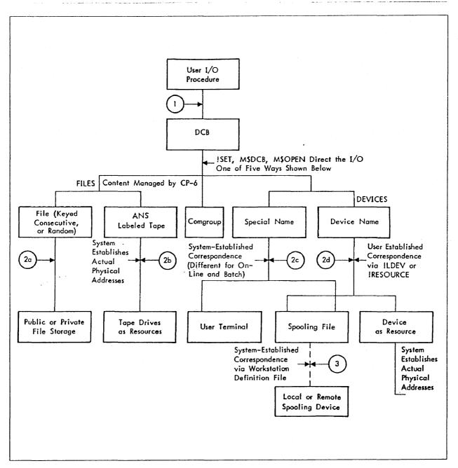
Figure 7-1. Connection Established for Performing I/O
