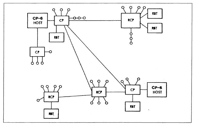
Figure 9–1. Sample CP-6 Communication Configuration
