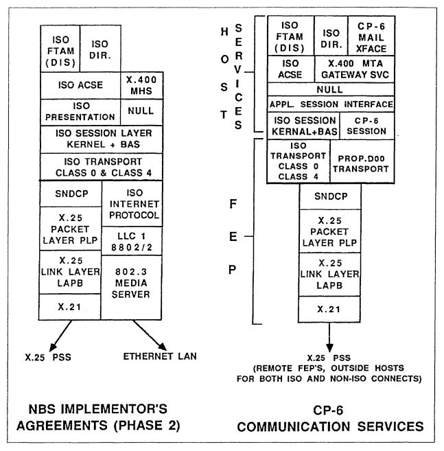
Figure 14–3. NBS and CP-6 Communication Models
