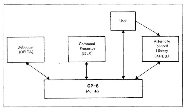
Figure 8-3. Control Paths Between CP-6 Working Spaces
