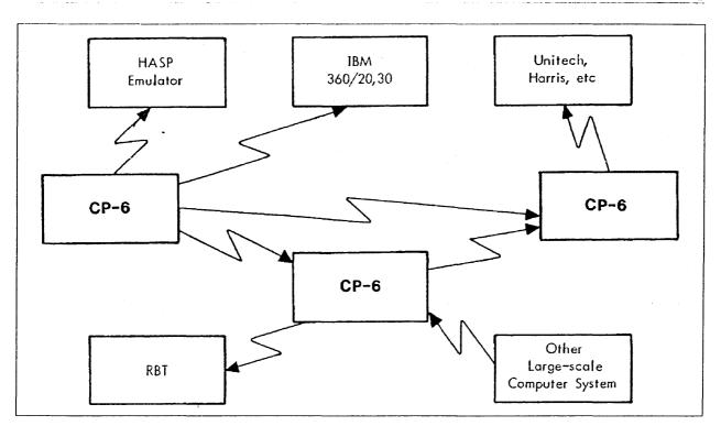
Figure 14–2. CP-6 Remote Processing Communications
