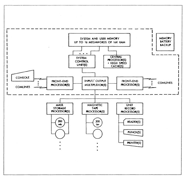
Figure 3–1. Generalized CP-6 L66 DPS Configuration
