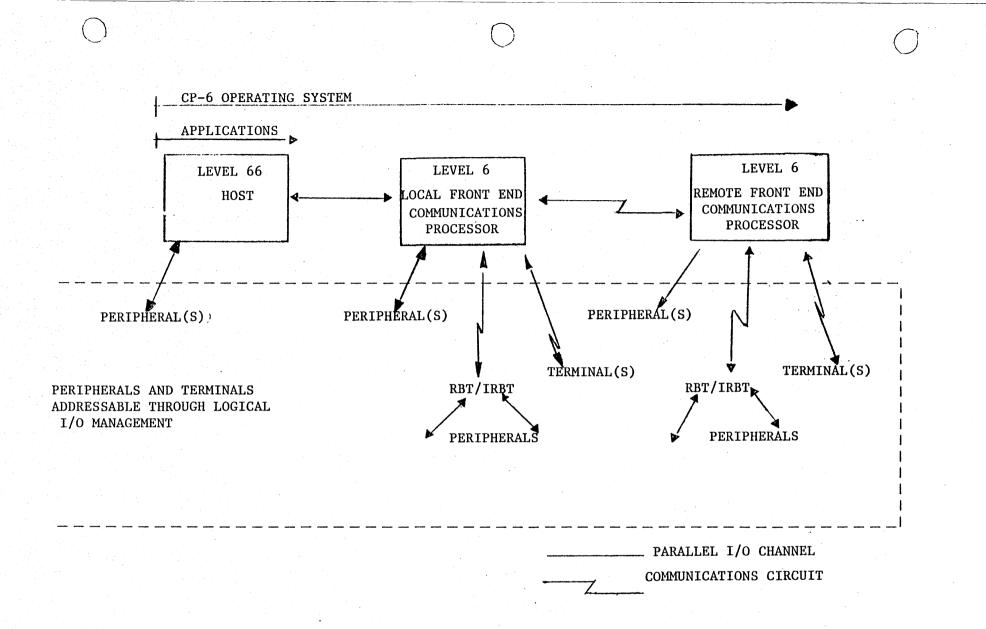
FIGURE 4.4.4.-1 HOST ADDRESSABLE PERIPHERAL UNITS
