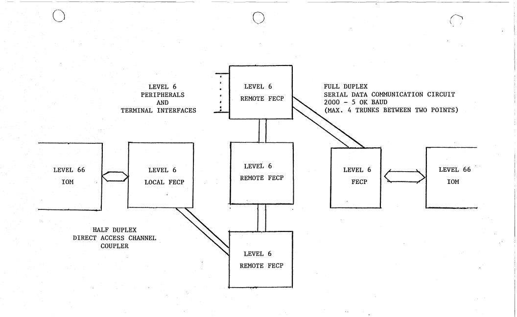
FIGURE 4.4.4.-2 FRONT END COMMUNICATIONS PROCESSORS
