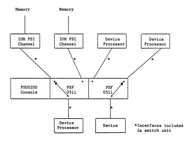
Figure 12-5. Switching Between Two Device Processors and Between Two IOM Physical Channels
