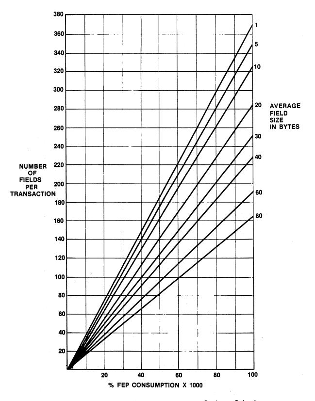
Figure 11-11. FEP TP Forms Performance, Systems Output (1000 Transactions Per Hour)
