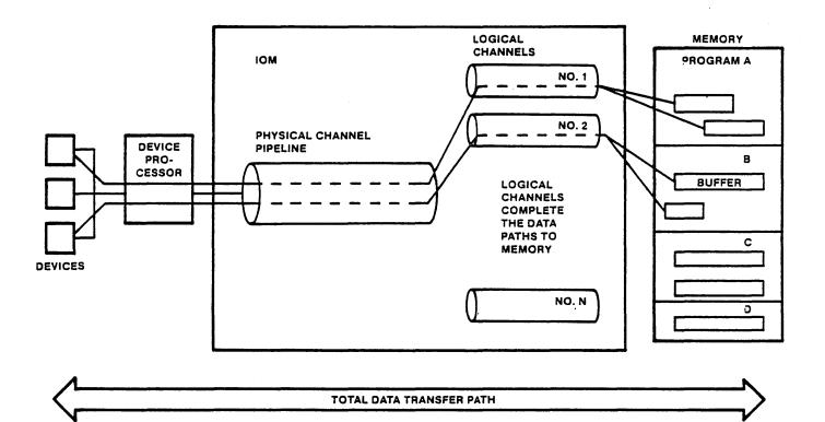
Figure 5-2. Physical Channel and Logical Channel Concepts
