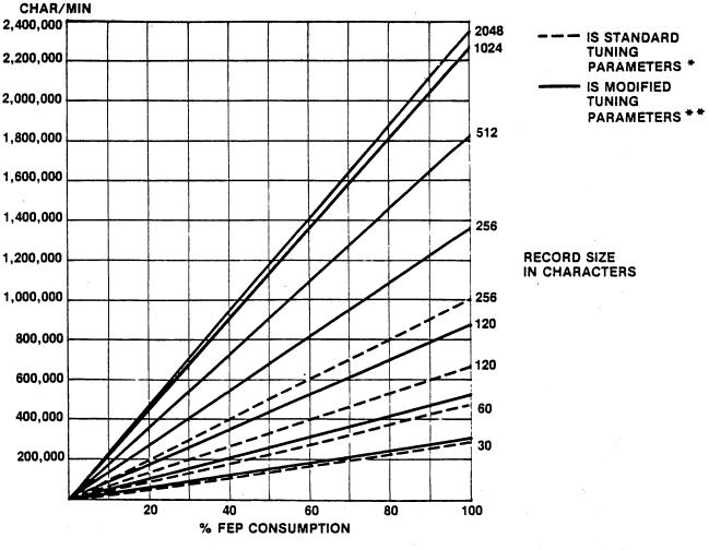
Figure 11-6. ASYNC Output Performance Transparent
