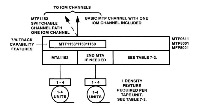
Figure 7-1. Single-Channel MTP Configurator
