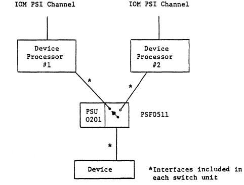
Figure 12-3. Switching Between Two Device Processors
