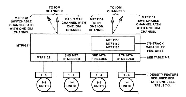
Figure 7-2. Dual-Channel MTP Configurator
