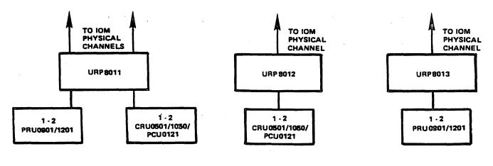
Figure 6-4. Configurators for URP8011/8012/8013
