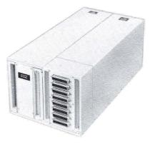
FIGURE 23. REAR VIEW OF COMPUTER. CENTRAL PROCESSOR UNIT All external connections are made through rack and panel connections on the rear of the units (see Figure 23). For ease of installation and adaptability to various systems, vibration isolation is not required except for the most stringent applications. Cooling may be either cold plate or forced air. Modular unit construction details will show that *ALERT* is designed to be reliable and easy to maintain.
