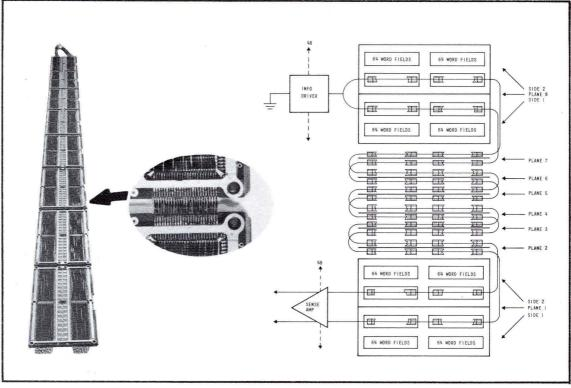
FIGURE 14. THE MEMORY STACK SHOWING SENSE WINDINGS.
