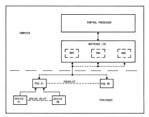
FIGURE 8. INFORMATION FLOW BETWEEN PERIPHERAL DEVICES AND ALERT.
