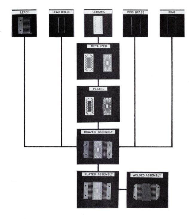
FIGURE 18. STEPS IN FLATPACK CONSTRUCTION.
