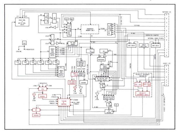
FIGURE 3. TIMING AND CONTROL LOGIC EMPHASIZED IN CENTRAL PROCESSOR.
