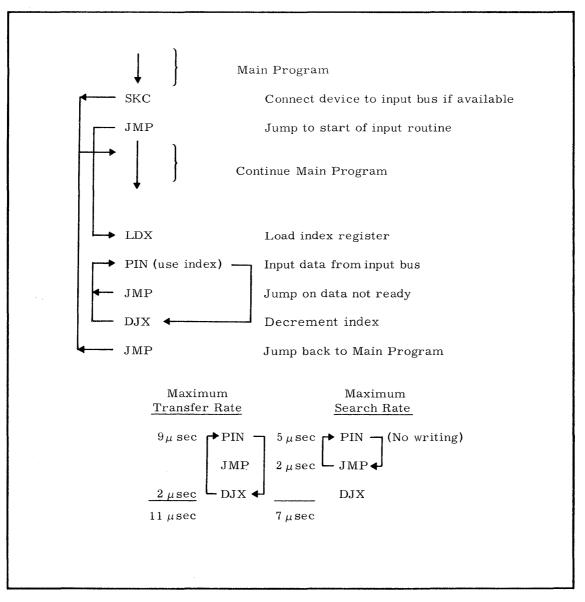
FIGURE 6. PROCEDURE AND RATE FOR MAXIMUM INPUT TRANSFER.
