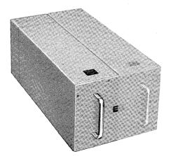
ALERT central processor is 5 inches by 7.6 inches by 19.5 inches and contains a direct input/output channel in addition to circuitry neccessary to perform arithmetic functions. Characteristics include:
