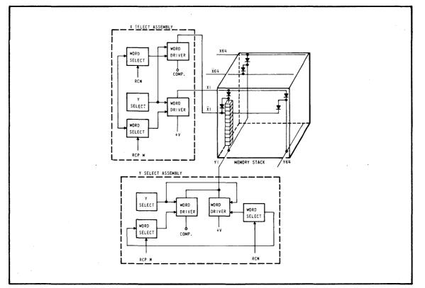
FIGURE 13. THE SELECTION MATRIX SHOWING X AND Y SELECT ASSEMBLIES.
