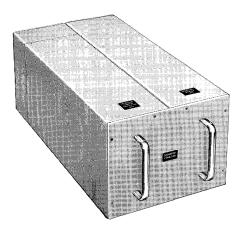
ALERT, in its basic configuration, consists of two separate modules interconnected to form one offthe-shelf general-purpose scientific computer.
