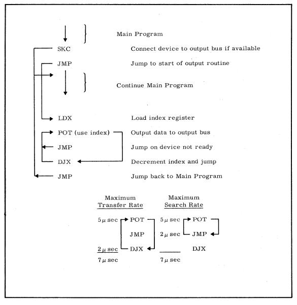
FIGURE 7. PROCEDURE AND RATE FOR MAXIMUM OUTPUT TRANSFER.
