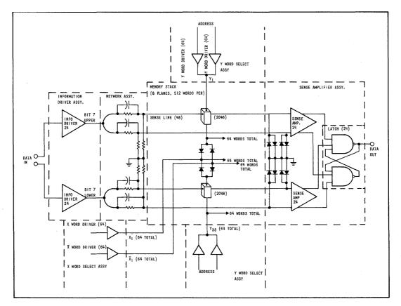
FIGURE 16. READ, WRITE, AND SELECTION SCHEME.
