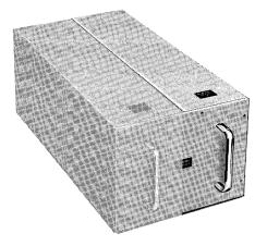
Memory modules vary in size according to number of words. The basic 4,096 word module is 5 inches by 7.6 inches by 19.5 inches and the fully expanded 32,768 word version increases width to 25.25 inches. Height and depth remain constant. Characteristics include:
