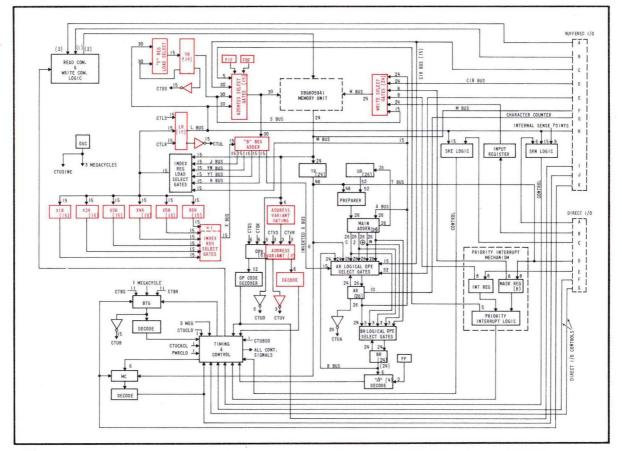
FIGURE 2. ADDRESSING LOGIC EMPHASIZED IN CENTRAL PROCESSOR.
