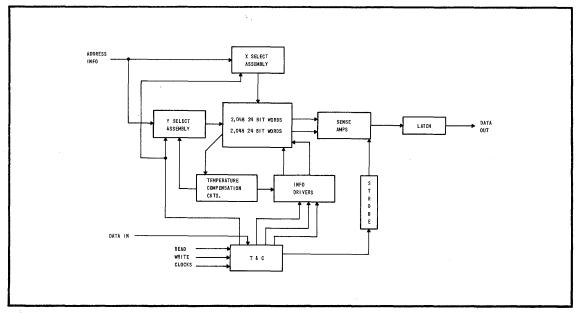
FIGURE 15. THE MEMORY STACK AND ASSOCIATED ELECTRONICS.
