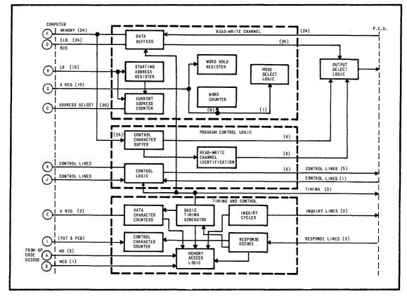
FIGURE 9. THE BUFFERED INPUT/OUTPUT CHANNEL.
