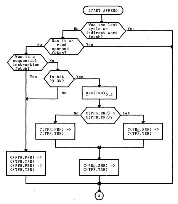
Figure 8-1. Complete Appending Unit Operation Flowchart
