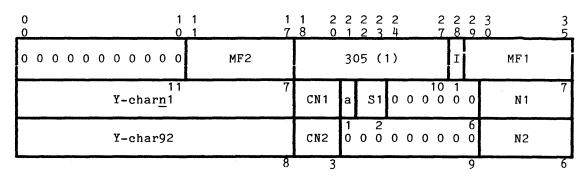
Figure 4-26. Decimal to Binary Convert (dtb) EIS Multiword Instruction Format
