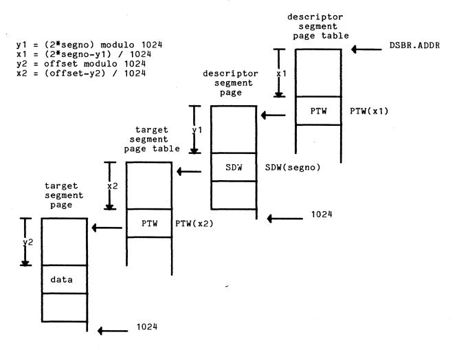
Figure 5-3. Main Memory Address Generation for Paged Segments
