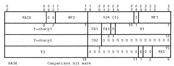
Figure 4-15. Scan with Mask (sem) EIS Multiword Instruction Format
