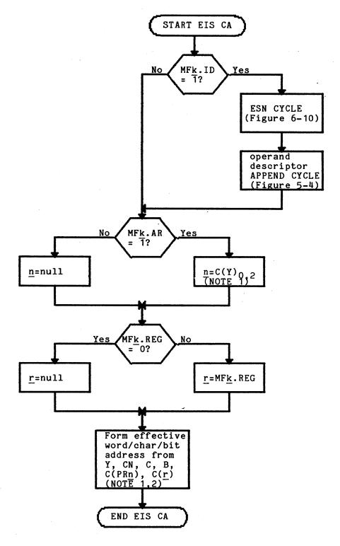
Figure 6-11. EIS Virtual Address Formation Flowchart
