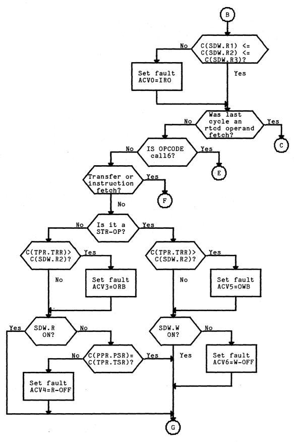
Figure 8-1(cont). Complete Appending Unit Operation Flowchart
