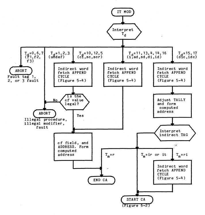
Figure 6-6. Indirect Then Tally Modification Flowchart
