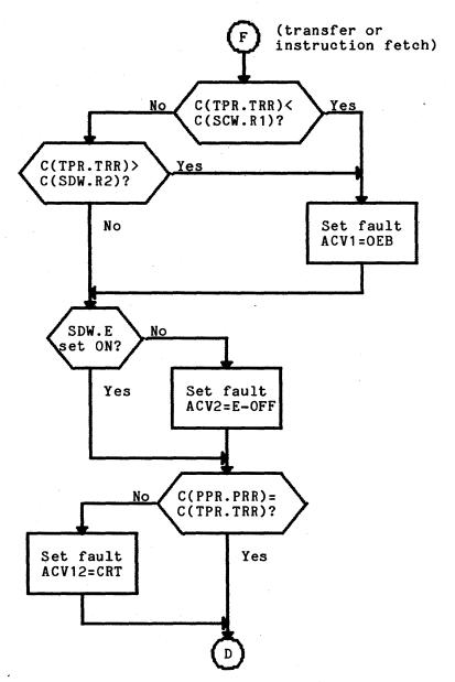
Figure 8-1(cont). Complete Appending Unit Operation Flowchart
