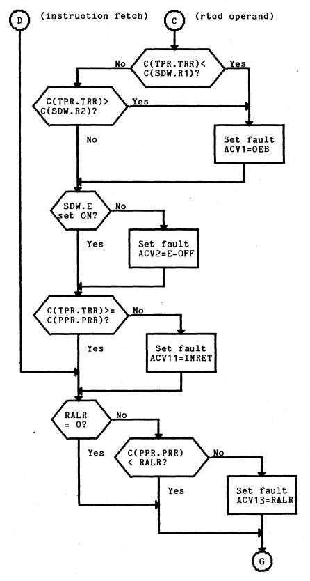
Figure 8-1(cont). Complete Appending Unit Operation Flowchart
