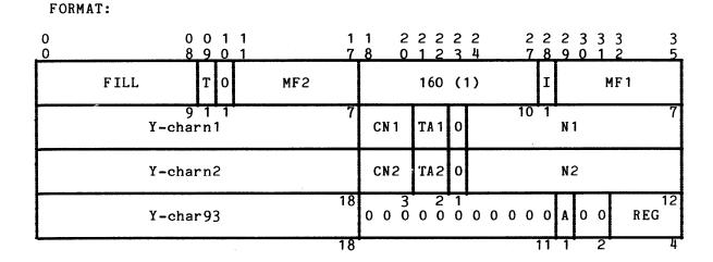
Figure 4-1. Move Alphanumeric with Translation (mvt) EIS Multiword Instruction Format
