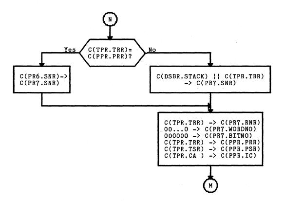
Figure 8-1(cont). Complete Appending Unit Operation Flowchart
