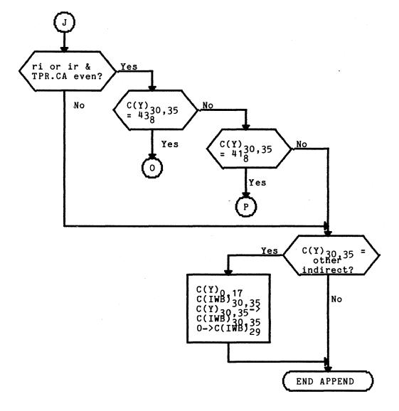
Figure 8-1(cont). Complete Appending Unit Operation Flowchart
