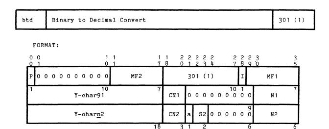
Figure 4-25. Binary to Decimal Convert (BTD) EIS Multiword Instruction Format
