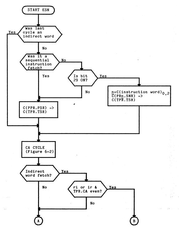
Figure 6-10. Effective Segment Generation Flowchart
