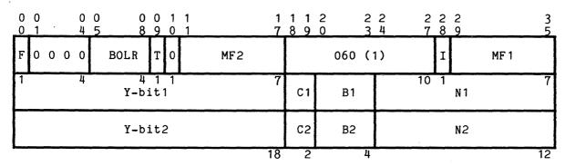
Figure 4-23. Combine Bit Strings Left (csl) EIS Multiword Instruction Format
