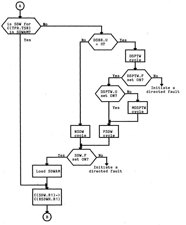
Figure 8-1(cont). Complete Appending Unit Operation Flowchart
