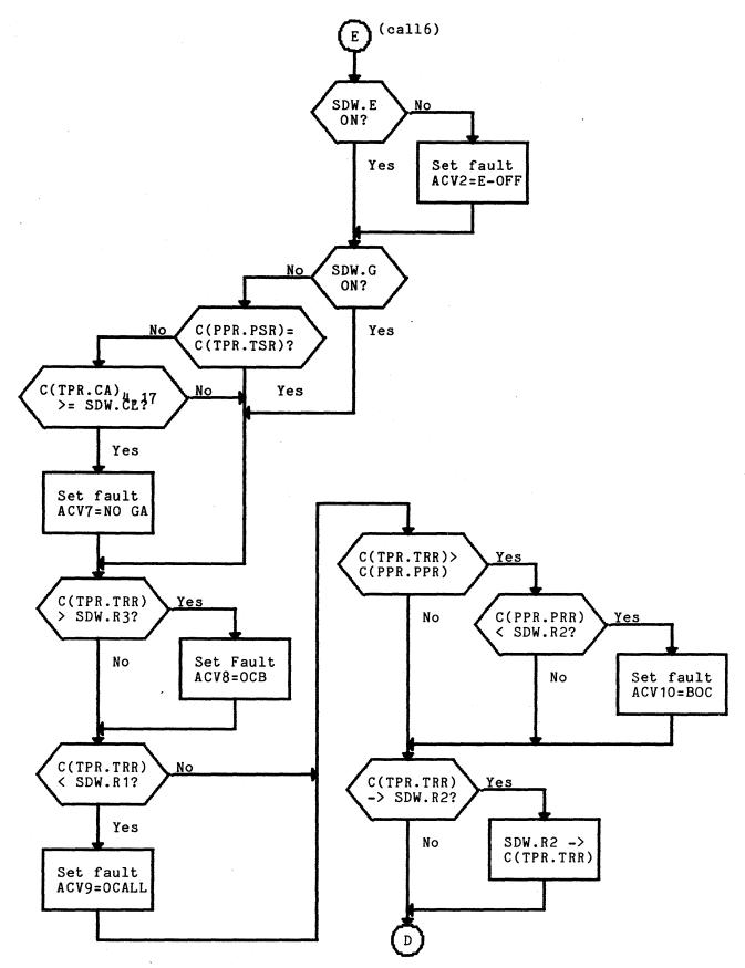
Figure 8-1(cont). Complete Appending Unit Operation Flowchart
