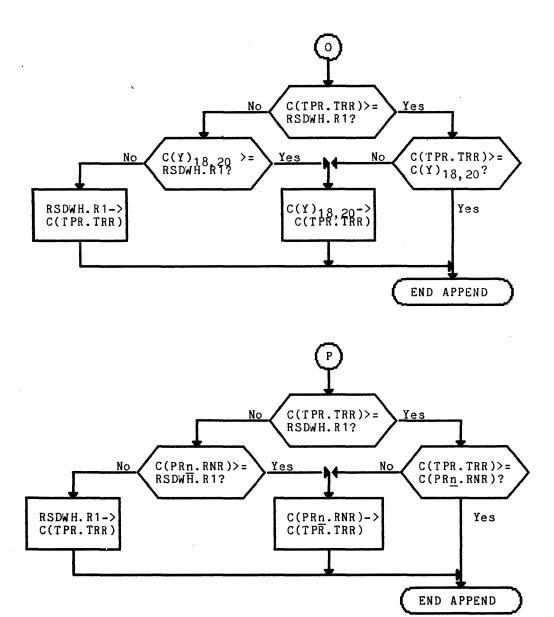
Figure 8-1 (cont). Complete Appending Unit Operation Flowchart
