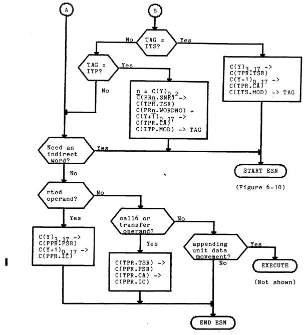
Figure 6-10(cont). Effective Segment Number Generation Flowchart
