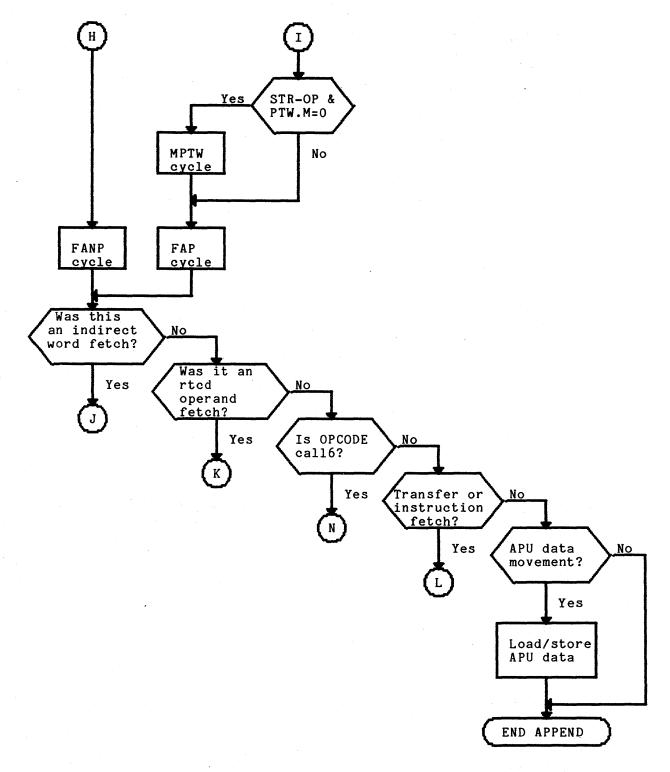
Figure 8-1(cont). Complete Appending Unit Operation Flowchart
