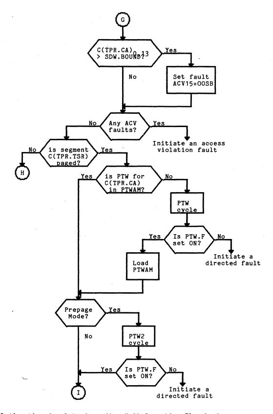
Figure 8-1(cont). Complete Appending Unit Operation Flowchart
