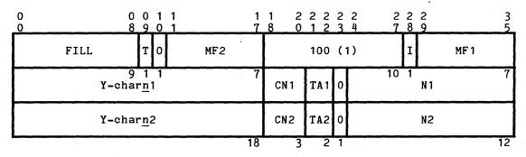
Figure 4-17. Move Alphanumeric Left to Right (mlr) EIS Multiword Instruction Format
