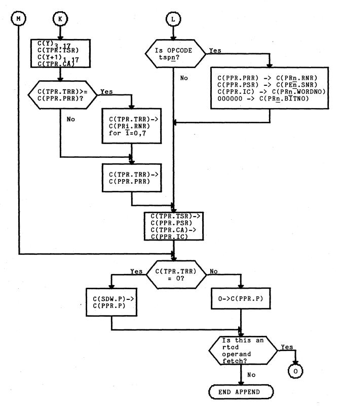
Figure 8-1(cont). Complete Appending Unit Operation Flowchart
