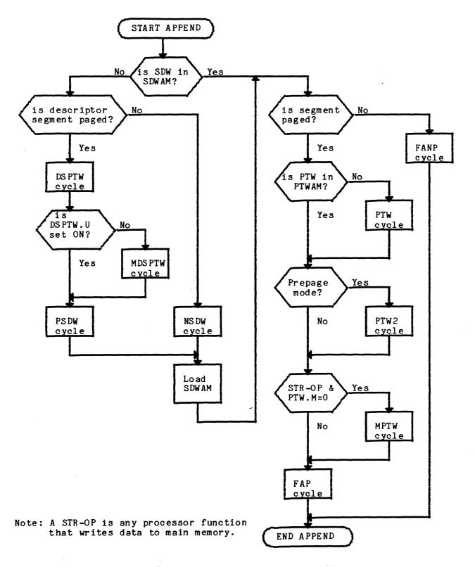
Figure 5-4. Appending Unit Operation Flowchart
