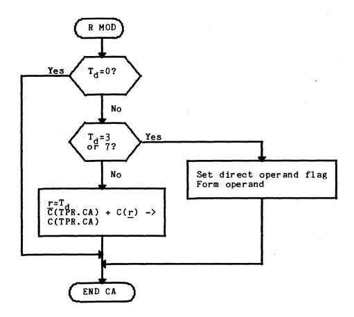
Figure 6-3. Register Modification Flowchart
