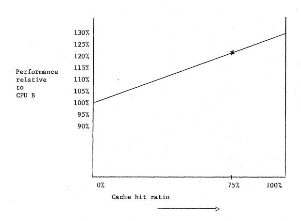
Figure 1 -- CPU A performance relative to CPU B, as a function of cache hit ratio.
