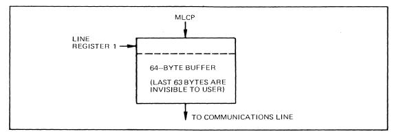
Figure E-8. Line Register 1 for Transmit Channel
