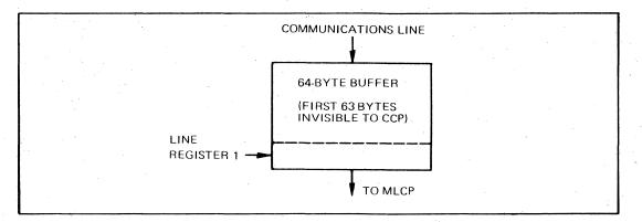
Figure E-3. Line Register 1 for Receive Channel
