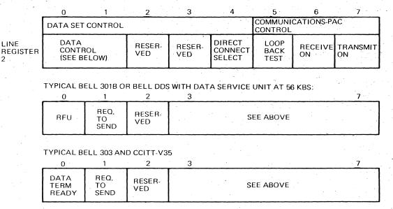
Line Register 2-Receive/Transmit Channel
