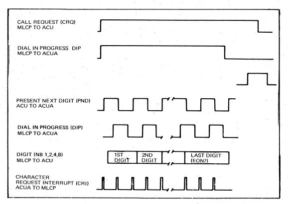
Figure F-7. Typical Automatic Calling Equipment/DCM9110/MLCP Timing Sequence
