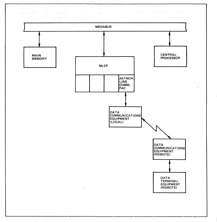
Figure C-1. Interface Provided by Asynchronous Line Communications-Pac (MLCP)
