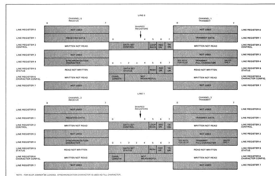
Figure D-3. Registers of Synchronous Line Communications-Pac/Adapter
