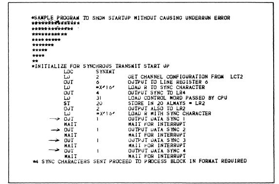
Figure D-4. Sample Program Showing Startup Without Causing Underrun Error (MLCP and DLCP)
