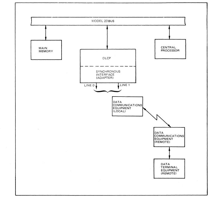
Figure D-2. Interface Provided by Synchronous Line Adapter (DLCP)
