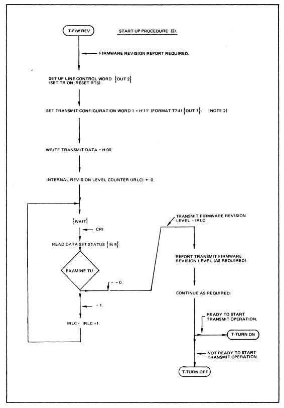
Figure H-18 (cont). Transmit Flowchart
