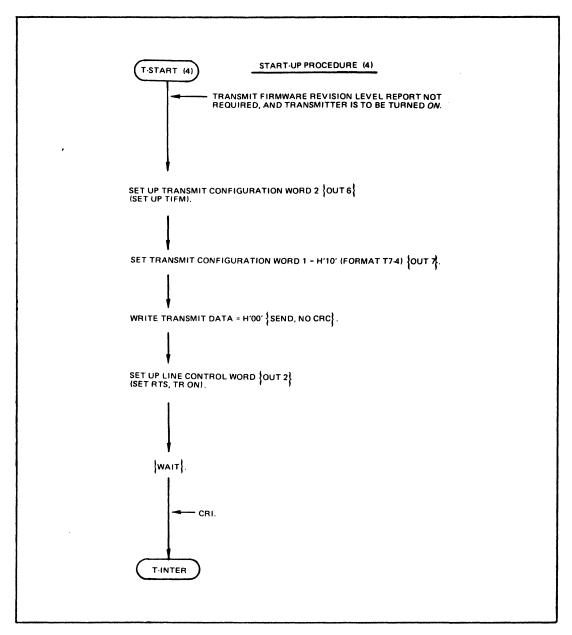
Figure H-18 (cont). Transmit Flowchart
