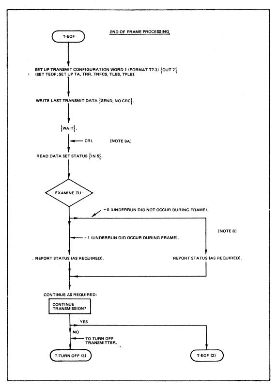
Figure H-18 (cont). Transmit Flowchart
