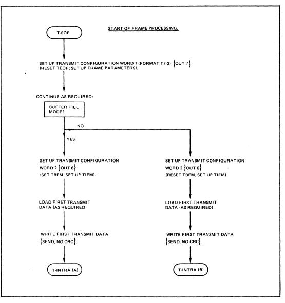
Figure H-18 (cont). Transmit Flowchart
