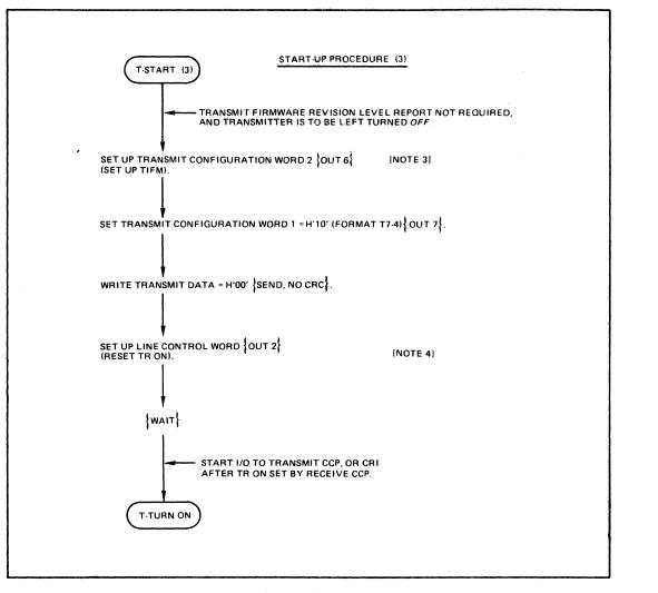
Figure H-18 (cont). Transmit Flowchart
