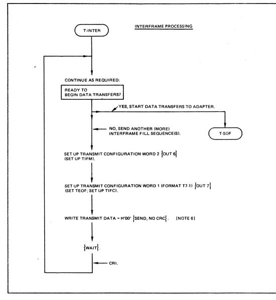
Figure H-18 (cont). Transmit Flowchart
