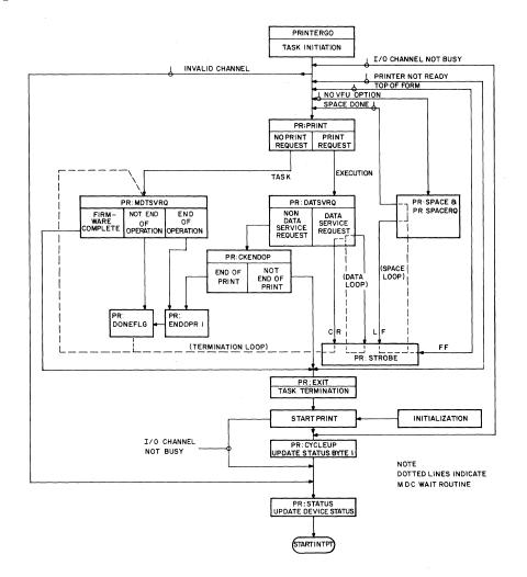
Figure 3-2 Functional Flow Chart for Printer Adapter Firmware
