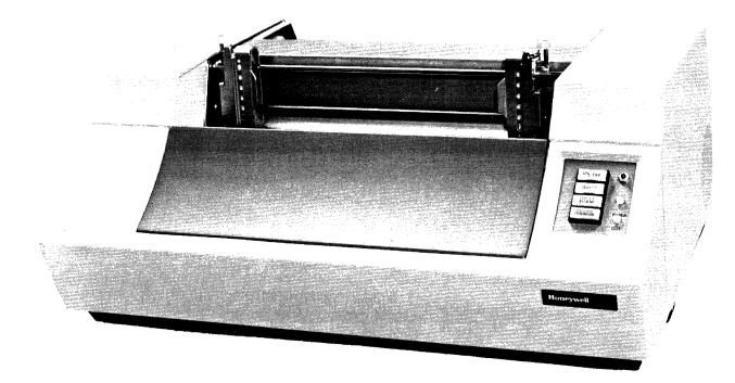
Figure 1-5 Serial Matrix Printer
