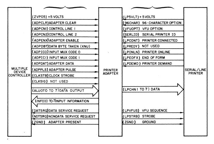
Figure 2-2 MDC/Adapter/Printer Interface
