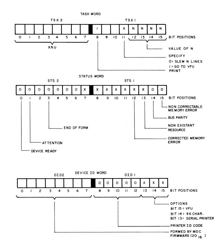
Figure 3-1 Device-Specific Word Bit Structures (Sheet 1 of 2)
