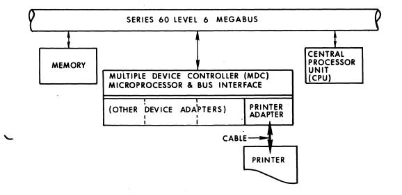
Figure 1-1 MDC, Printer Adapter, and Printer Interface
