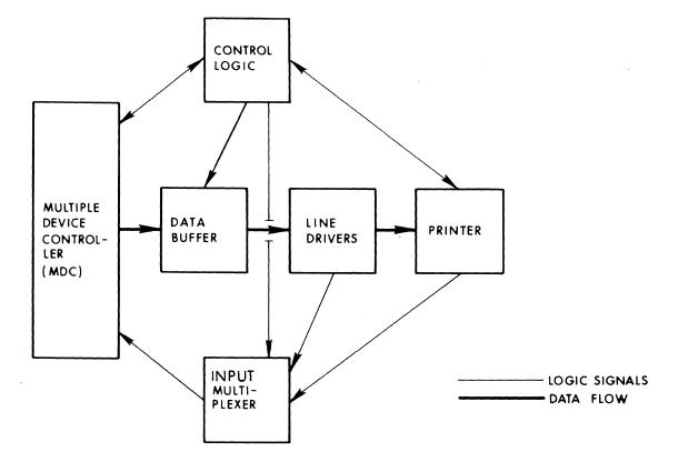
Figure 1-2 Data Flow Through Printer Adapter
