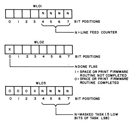
Figure 3-1 Device-Specific Word Bid Structures (Sheet 2 of 2)
