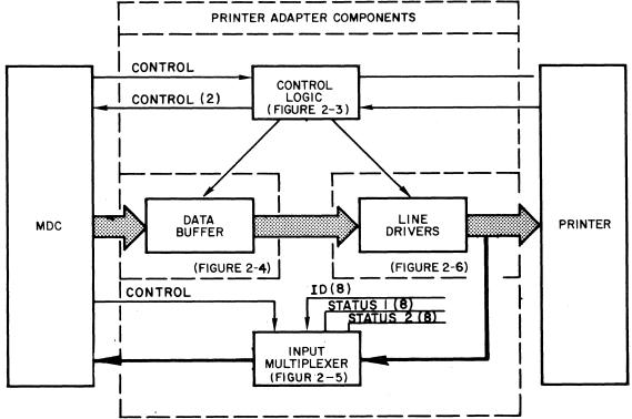
Figure 2-1 Printer Adapter, Major Block Diagram
