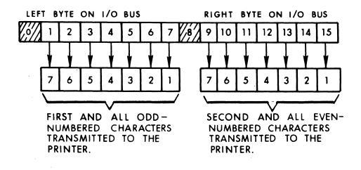
Figure 1-3 Data Transfer to Printer
