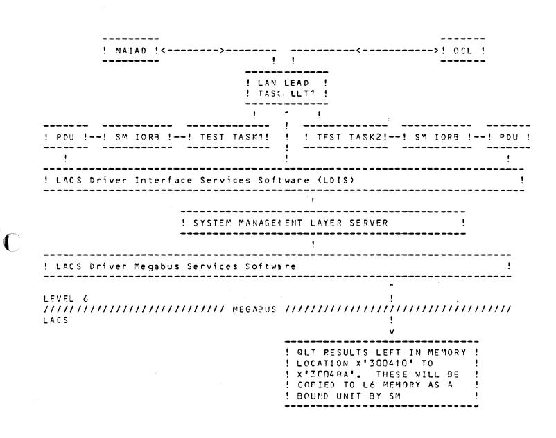
Figure 1 Operational Relationships between the Lan Test and the various Network Administration Layers during controller tests.
