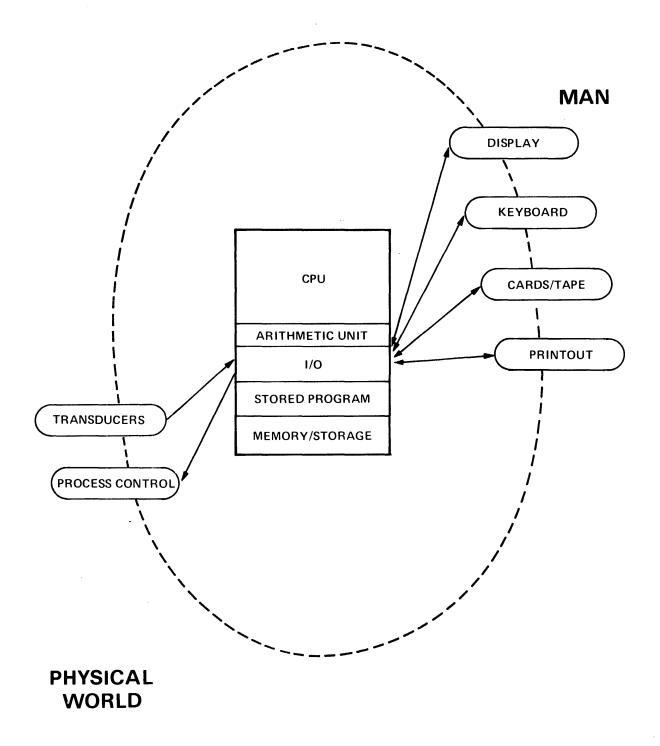
Inputs for this type of service include manual input on a keyboard, punched cards or tape. These can be on-line or off-line depending on the speed or convenience desired, and the operating system available. If tables or data are required, they may be provided on mag tape, disc or other suitable means.
