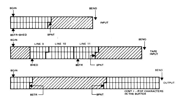
FIGURE 13. INPUT/OUTPUT BUFFERING
