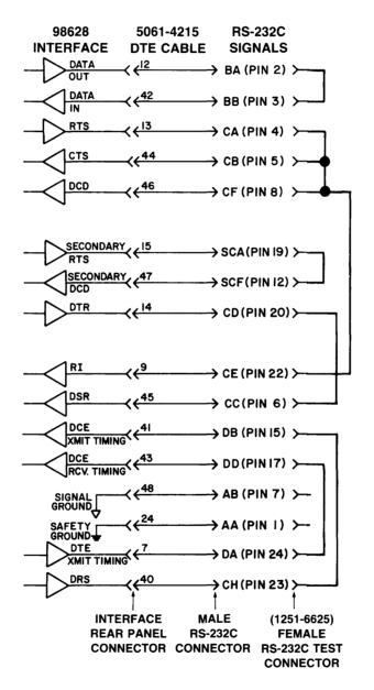
**Option 001 DTE Interface Cable and Test Connector**
