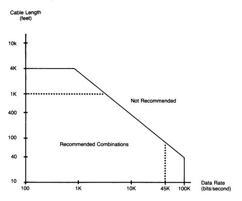
**RS-423 Modulation Rate Versus Cable Length**
