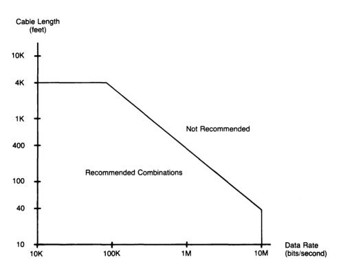
**RS-422** Modulation Rate Versus Cable Length
