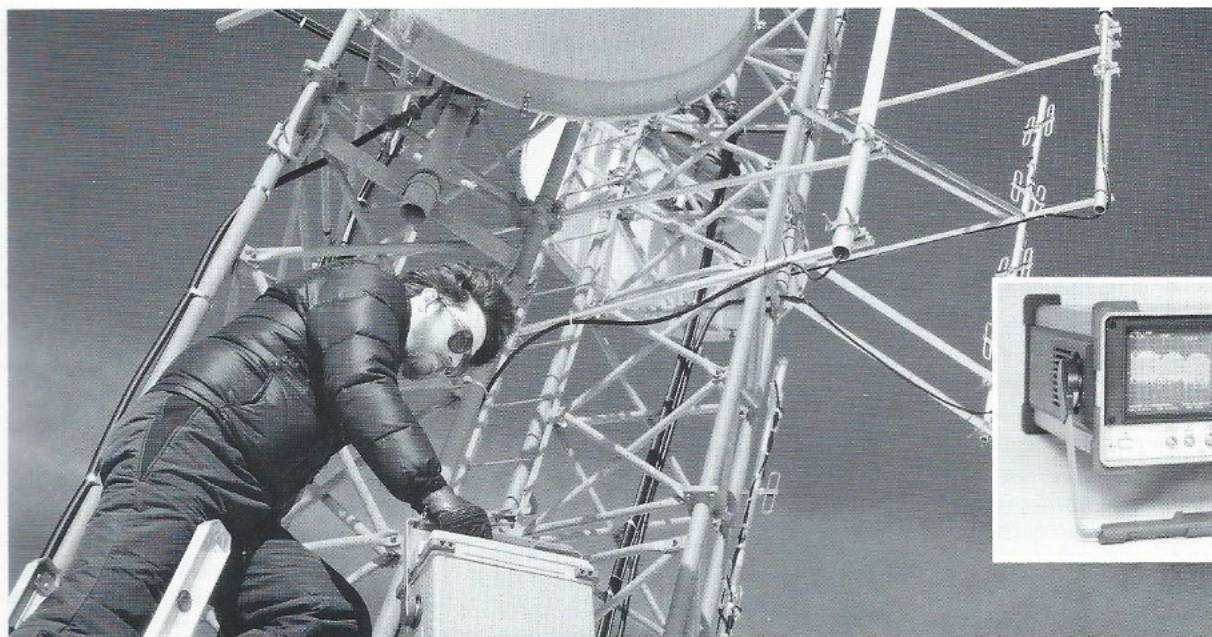
The new HP 8562A/B Portable Spectrum Analyzers (1 kHz-22 GHz) feature synthesized tuning, built-in AM/FM demodulators
