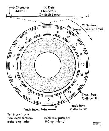
Figure 3. Arrangement of Data on a Disk
