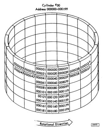
Figure 4. Addressing for Cylinder 00
