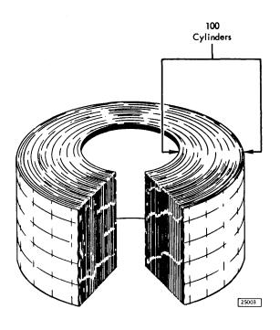
Figure 2. Cylinder Concept
