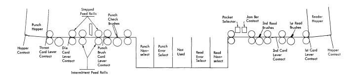
Figure 11. 1622 Feed Schematic
