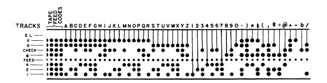
Figure 9. Paper Tape Tracks and Codes
