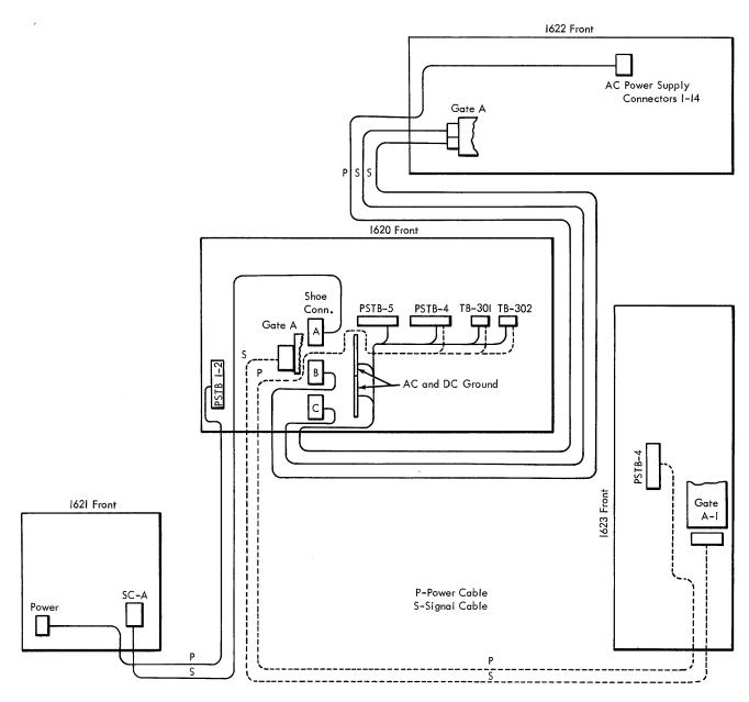
Figure 6. IBM 1620 Cable Connectors
