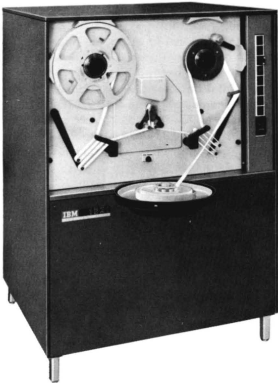
Figure 1. 1621 Paper Tape Reader
