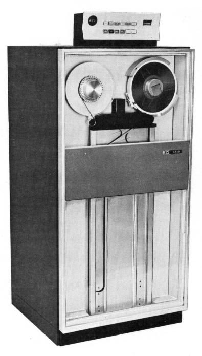
IBM 2420 Model 7 Magnetic Tape Unit
