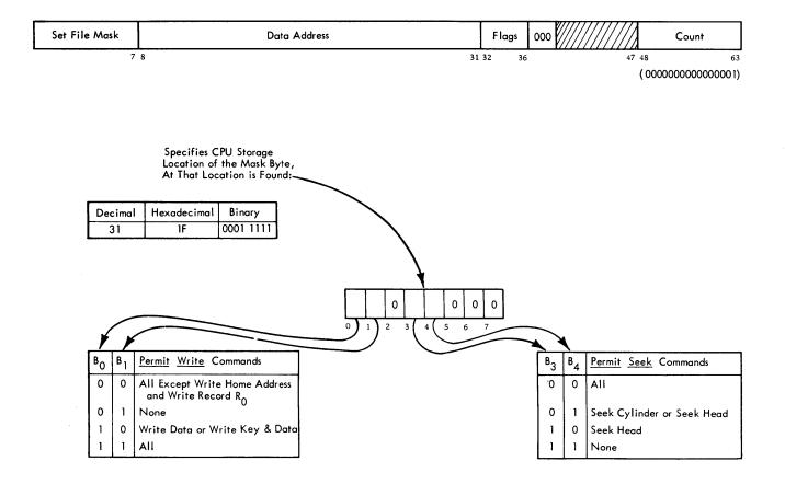
For the 2841 Storage Control, B2, B5, B6, and B7 of the mask must be zero. If these bits are not zero, the mask is considered to be invalid and a CSW Unit Check signal is generated. A subsequent Sense I/O command will indicate Command Reject.
