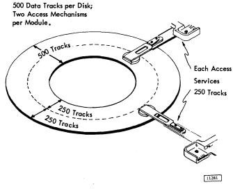
Figure 15. Access Mechanisms
