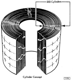
Once the access mechanism has reached a cylinder position, additional time is required for disk rotation to the desired record. At 2,400 revolutions per minute, rotation time is 25 ms, and one-half revolution (12.5 ms) is the average rotational delay.
