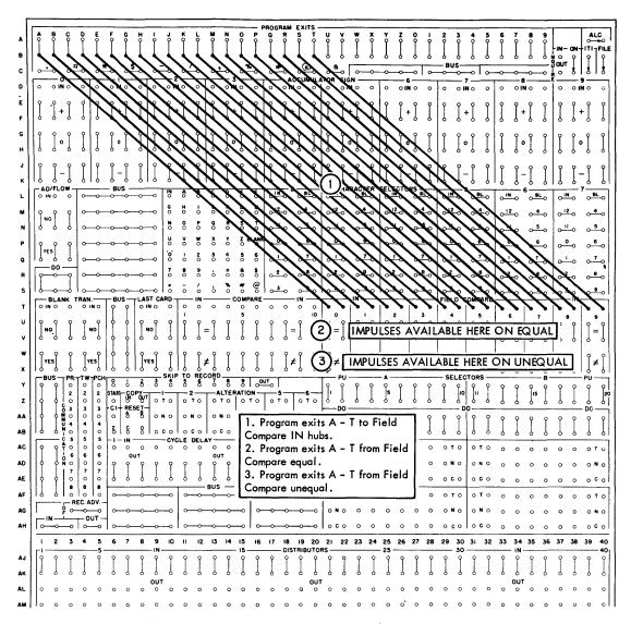
Figure 119. Program Exit Expansion-Field Compare Selectors
