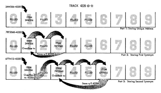
Figure 42. Chaining Method of Loading the File
