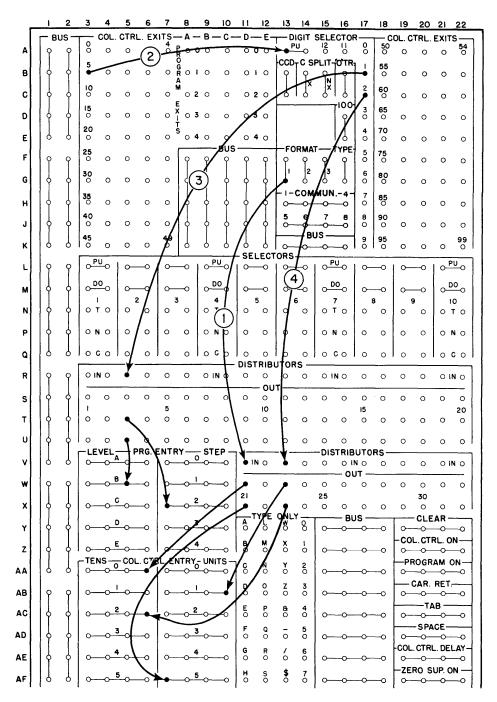
Figure 67. Alteration of Format Control
