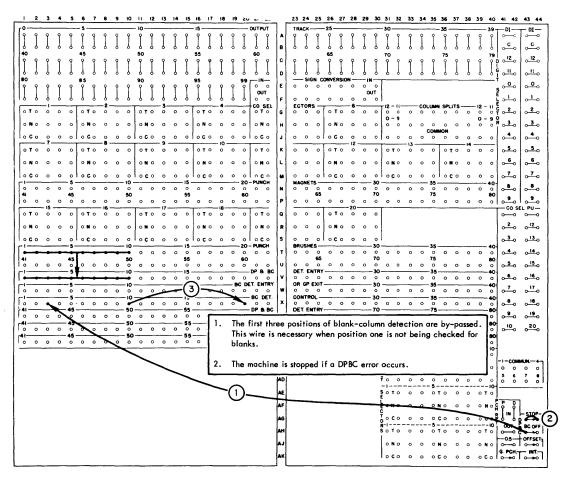
Figure 111. Double-Punch and Blank-Column Detection
