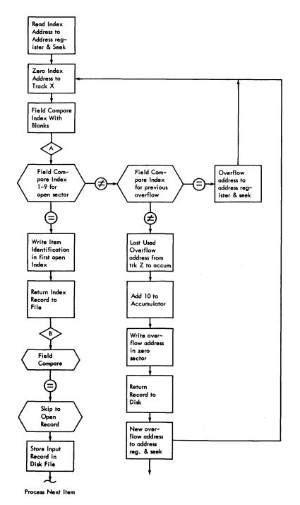
Figure 37. Constructing an Index Record and Storing a Record (Block Diagram)
