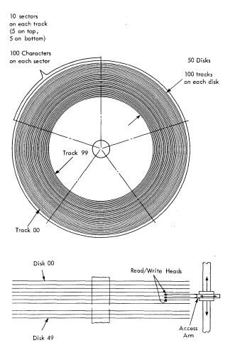
Figure 4. Schematic Disk Storage
