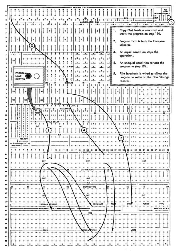
Figure 30. Control Panel Wiring for Clearing Disk Storage
