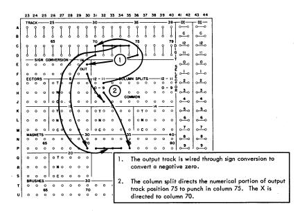
Figure 107. Punch Negative X over High-Order Position
