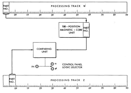
Figure 18. Schematic of a Comparing Operation
