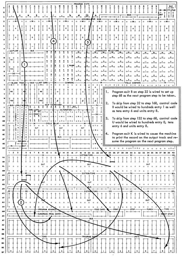
Figure 11. Method of Wiring Program Transfers
