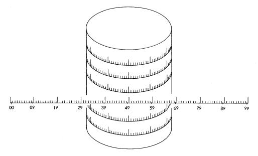
Figure 8. Graphic Representation of Drum Tracks
