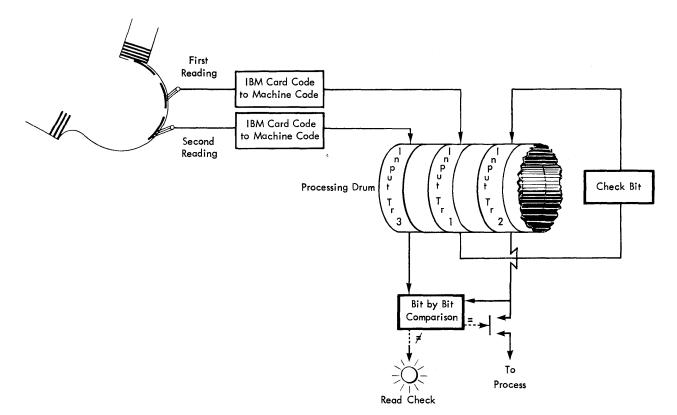
Figure 47. Checking of Input Card Reading
