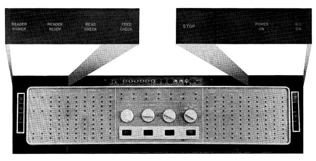
Figure 56. Power, Machine Stop and Reader Lights
