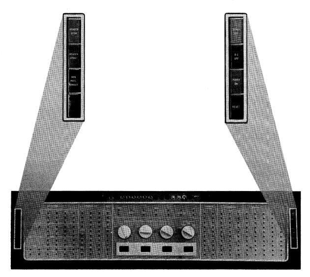
Figure 53. Power, Reset and Reader Keys
