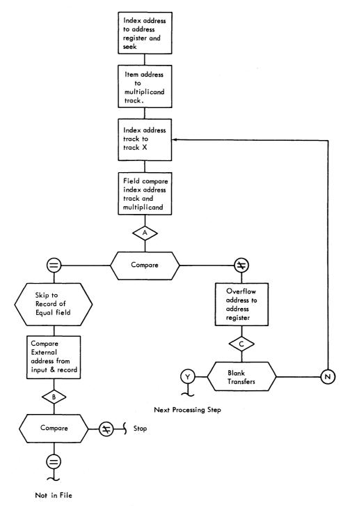
Figure 40. Locating a Record During Processing
