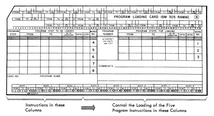
Figure 12. Card Used for Program Loading
