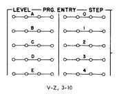
Program Entry. To establish the beginning of a sequence of program impulses, one LEVEL hub and one STEP hub are impulsed in the same manner that the PRO-GRAM ENTRY hubs are impulsed on the process control panel. The program unit is turned on automatically by impulsing PROGRAM ENTRY, without impulsing PROGRAM ON.
