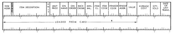
Figure 31. Track Layout of an Item in Disk Storage
