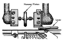
Figure 92. Printer Platen
