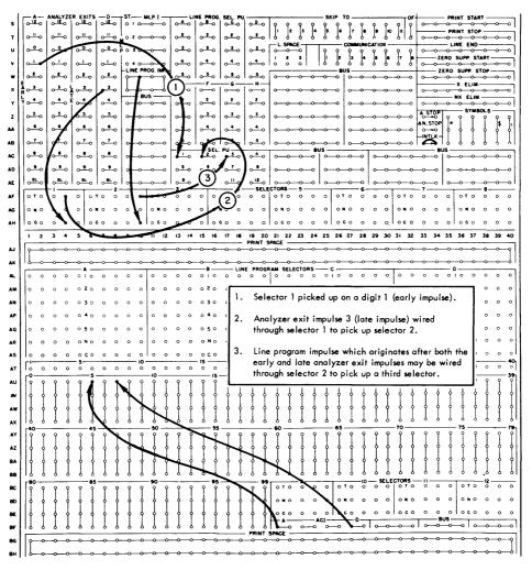
Figure 100. Series Wiring to Illustrate Timings
