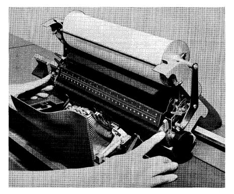
Figure 73. Removing the Platen
