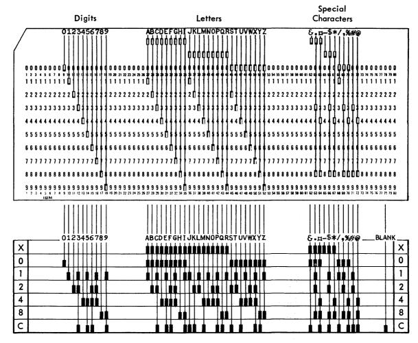
Figure 46. Character Coding for IBM Punched Card and IBM 305 RAMAC
