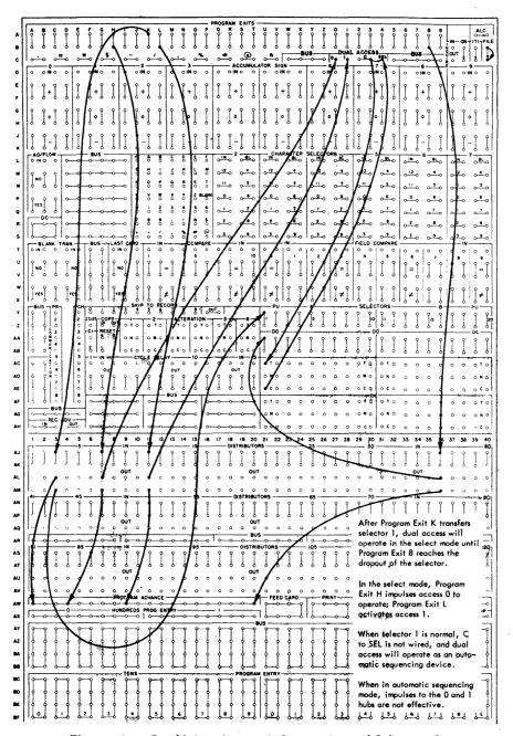
Figure 140. Combining Automatic Sequencing and Select Mode
