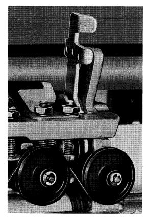
Figure 91. Forms Thickness Adjustment Device
