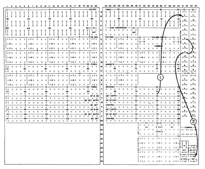
Figure 128. Off-setting Different Types of Cards
