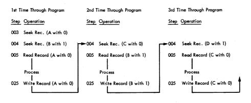
The first seek instruction following a reset condition will be directed automatically to the 0 access unit. On the next seek instruction in the program, access 1 will seek the address sent to the address register and access unit 0 will be conditioned to read or write. Therefore, the next read or write instruction issued will apply to access 0.
