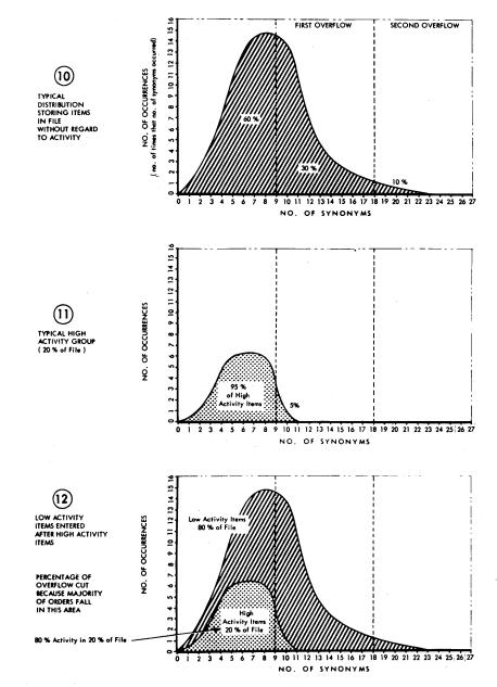
Figure 45. Typical Curves Obtained Using 80-20 Rule
