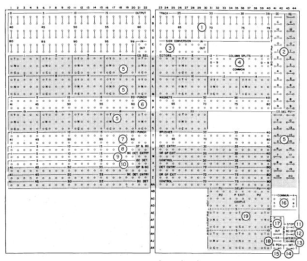
Figure 144. 323 Punch Control Panel
