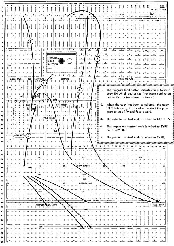
Figure 16. Control Panel Wiring for Loading the Program
