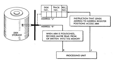
Figure 17. Method of Addressing, Reading and Writing in Disk Storage
