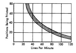
Figure 148. 370 Printer Speeds
