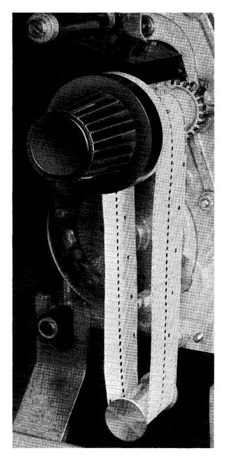
Figure 88. Forms Tractor Positioning Knob
