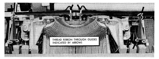
Figure 72. Typewriter Ribbon
