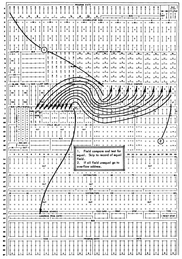
Figure 41. Locating a Record During Processing
