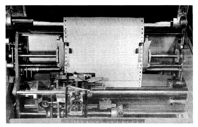
Figure 83. Tape-Controlled Carriage
