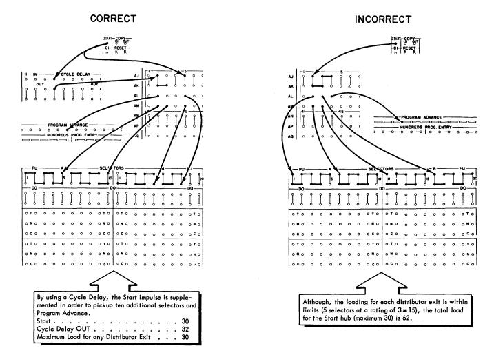
Figure 115. Wiring Based Upon Load Chart Ratings
