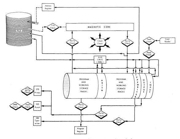
Figure 50. Summary of Automatic Machine Checks
