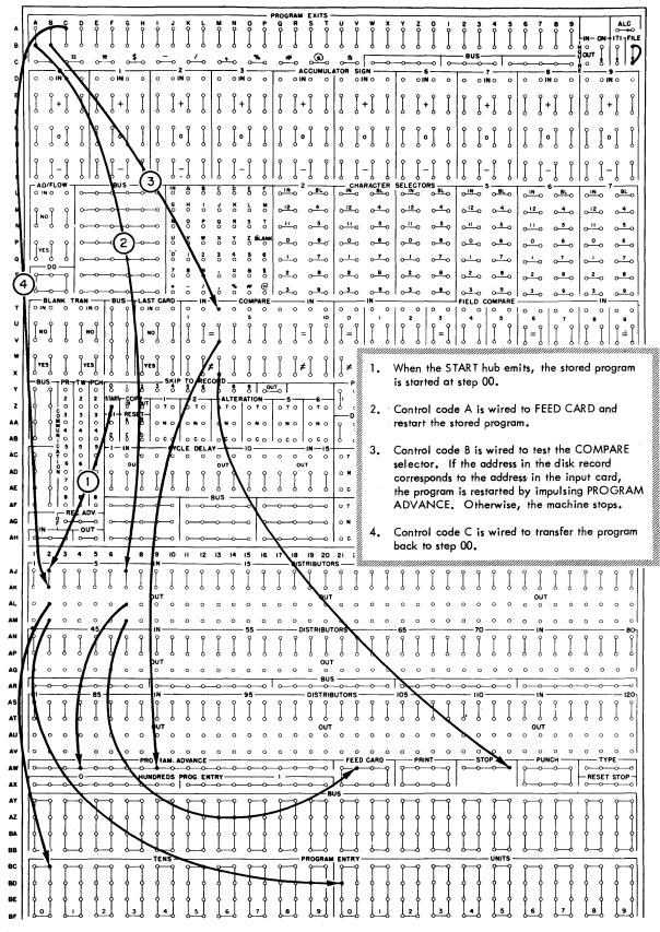
Figure 33. Control Panel Wiring for Loading Disk Storage
