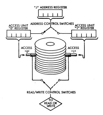
Figure 136. Schematic of Dual Access Units
