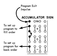
Figure 7. Method of Branching by Control Panel Wiring
