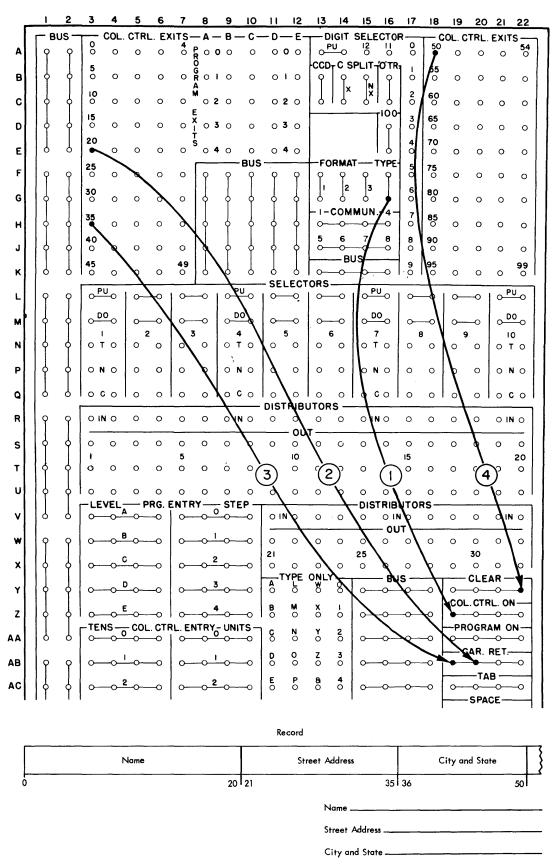
Figure 63. Printing a Three-Line Address
