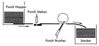
Figure 103. Punch Feed Schematic
