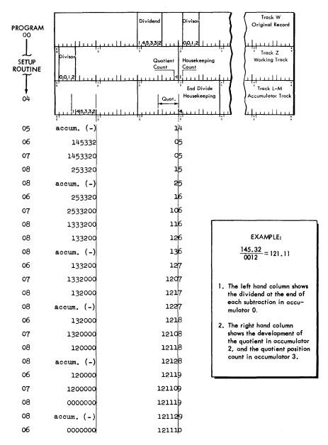
Figure 27. Division by Successive Subtraction (Example)
