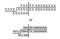
2. Note that the divisor must be positioned two places to the left on the multiplicand track, so that the first quotient digit will not exceed 9.
