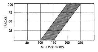
Figure 146. Seek Time for Access Arm moving from one track to another track on same disk
