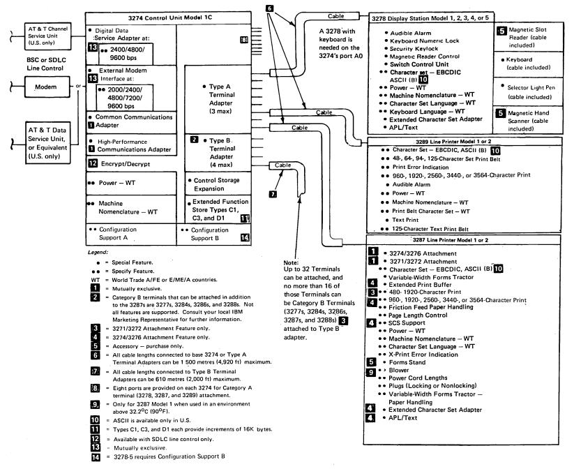
Figure 5-2. Configuring the 3278 Display Station Model 5, 3287 Printer Model 1 or 2, and 3289 Line Printer Model 1 or 2 on a Remotely Attached 3274 Control Unit Model 1C (BSC or SDLC Application)
