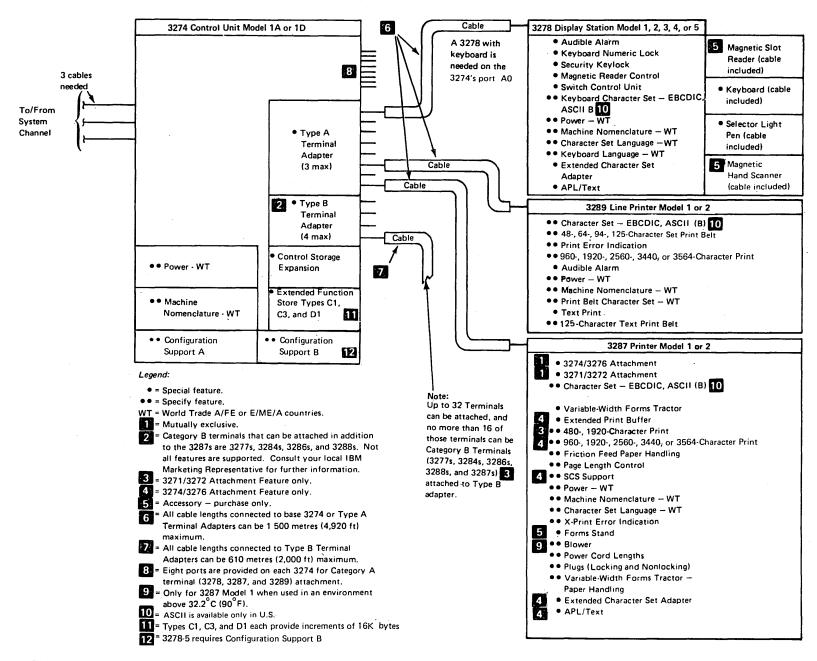
Figure 5-1. Configuring the 3278 Display Station Model 5, 3287 Printer Model 1 or 2, and 3289 Line Printer Model 1 or 2 on a Locally Attached 3274 Control Unit Model 1A or 1D
