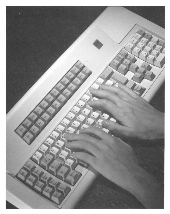
Figure 5-1. IBM 3270 Personal Computer Keyboard
