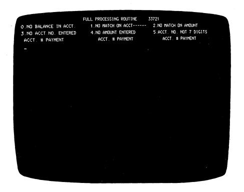
Figure 4-1. Displays Appearing during Sample Accounting Procedure (Display 1 of 3)
