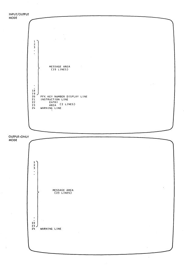
Note: These diagrams indicate how the display-screen lines are used in the two modes of operation; the labels shown do not appear on the screen.
