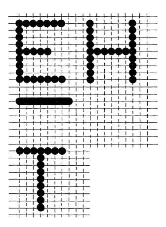
Figure 7-1. Examples of Monocase Characters Formed with 7 x 9 Dot Pattern
