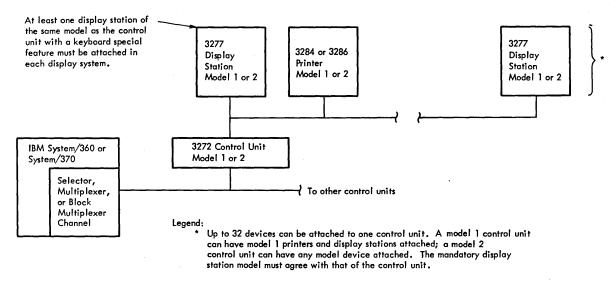
Figure 2-1. Locally Attached 3270 Display System
