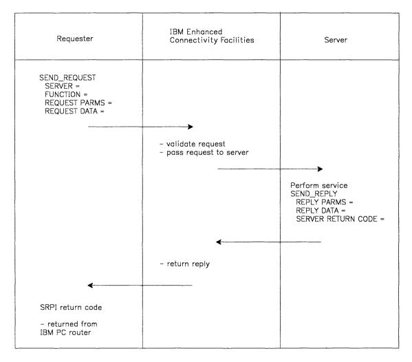
Figure 1-3. Example of a Requester and Server Flow
