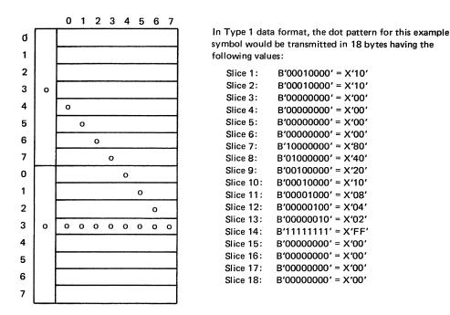
Figure J-1. Type 1 Data Format - An Example Dot Pattern Encoded
