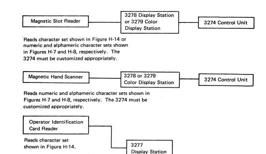
Figure H-3. Attachment of Magnetic Reading Devices to 3270 System Units
