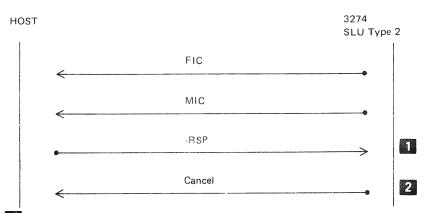
The type 2 SLU receives -RSP to a chain element. Note: Normally, the 3274 will not examine any response until the entire chain has been sent and will therefore not send Cancel as the result of receiving a -RSP. However, when inbound pacing is in effect, responses are examined when the SLU must receive a pacing response before continuing transmission. A -RSP will then be detected and cause Cancel to be sent.
