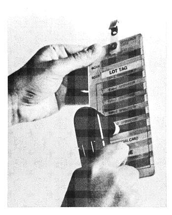
Figure H-5. Magnetic Hand Scanner (3278 and 3279 Attachments)
