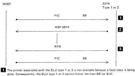
The SLU type 1 or 3 rejects BB (or Bid) with -RSP X'0814' (Bracket Reject, RTR to follow).
