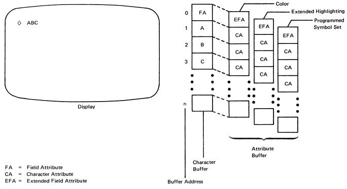
Figure 6-3. Model for Field Attributes and Extended Field Attributes, A Conceptual View
