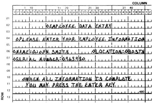
Figure 6-41. Data Entry Panel with Entered Data
