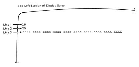
where xxxx xxxx ... represents the 20 bytes of data (x = 1 byte). From left to right, the data is interpreted as follows:
