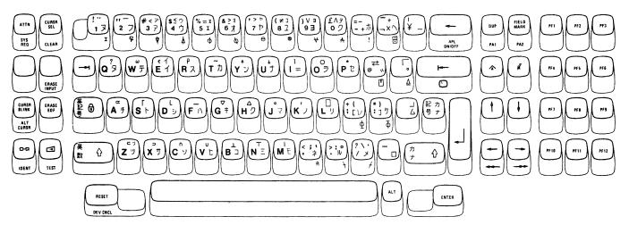
Figure D-9. 88-Key Katakana Typewriter/APL Keyboard
