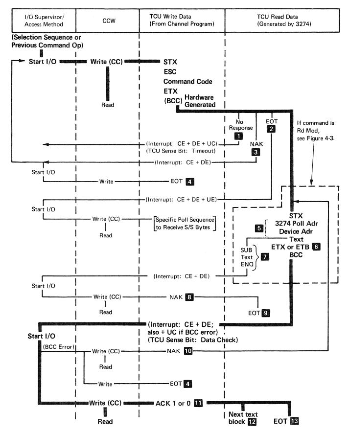
Figure 4-6 (Part 1 of 2). Read-Type Command, Sequence/Response Diagram
