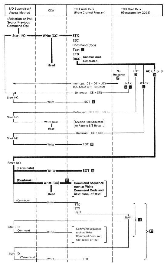
Figure 4-5 (Part 1 of 2). Write-Type and Control-Type Commands, Sequence/Response Diagram
