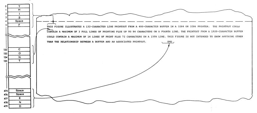
Figure 2-12. Relationship between Buffer Data and Printed Data
