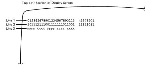
Line 1: Low-order digit of the port addresses configured on the 3274. When a Type B adapter is attached, the last (highest) Type A port and the first (lowest) Type B port are separated by two spaces on lines 1 and 2. The example shows 24 Type A terminals and eight Type B terminals.
