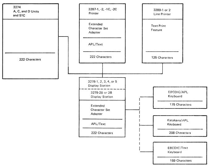
Figure D-1. Diagram of APL/Text Devices
