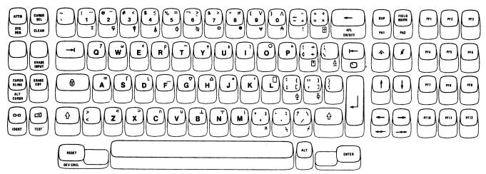
Figure D-8. 87-Key Typewriter/APL Keyboard
