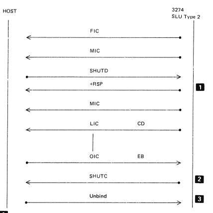
The SLU type 2 is alerted that the host wants to shut down. However, a synchronizing EB must be received before effecting shutdown.
