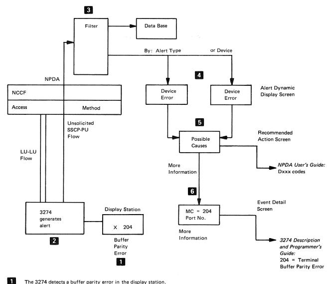
The 3274 detects a buffer parity error in the display station.
