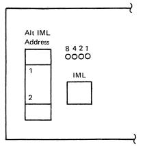
When the IML pushbutton is pressed, these lights are tested (they should all be on). When the IML pushbutton is released (or when the 3274 is initially powered on) the 3274 IML procedure is initiated.
