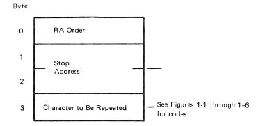
The third character following the RA order is always interpreted as the character that will be repeated. If an invalid stop address is specified, the write operation is terminated at this point without storing the character, and error status is generated. When Color, Extended Highlighting, or Programmed Symbols attributes are specified for the character, the attribute values are entered into the character attribute buffer as each repeated character is written in the data buffer.
