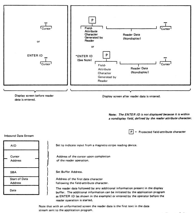
Figure H-16. Operation of the Display with an Unformatted Screen (OICR or MSR Using 3277-Compatible Numeric Character Set)
