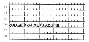
You must also place the location code at location R6, C36. You could use blanks after the name and an SBA sequence, or EUA with its associated address. Use PT instead. Insert a PT order after the "S" in "AMES". The single PT order clears the remainder of the unprotected name field to nulls and positions for the location code. PT should also follow the location code to position for the serial number. The data stream might look like this:
