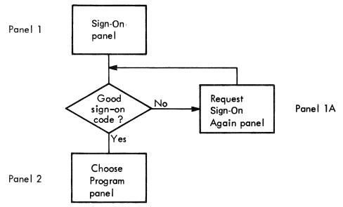
Figure 6-7. Block-Diagramming a Sequence of Panels
