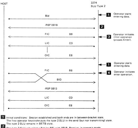
The type 2 SLU will reject a Bid (or BB) with 081B. Receiver in transmit mode.
