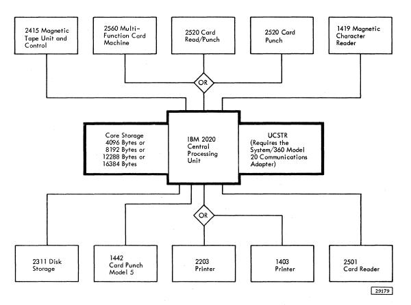
Figure 3. IBM System/360 Model 20 Units
