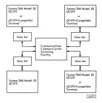
Figure 1. Point-to-Point Configuration
