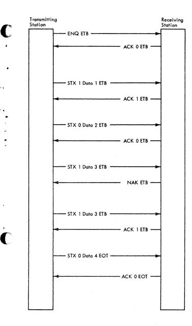
Figure 10. Message and Acknowledgment
