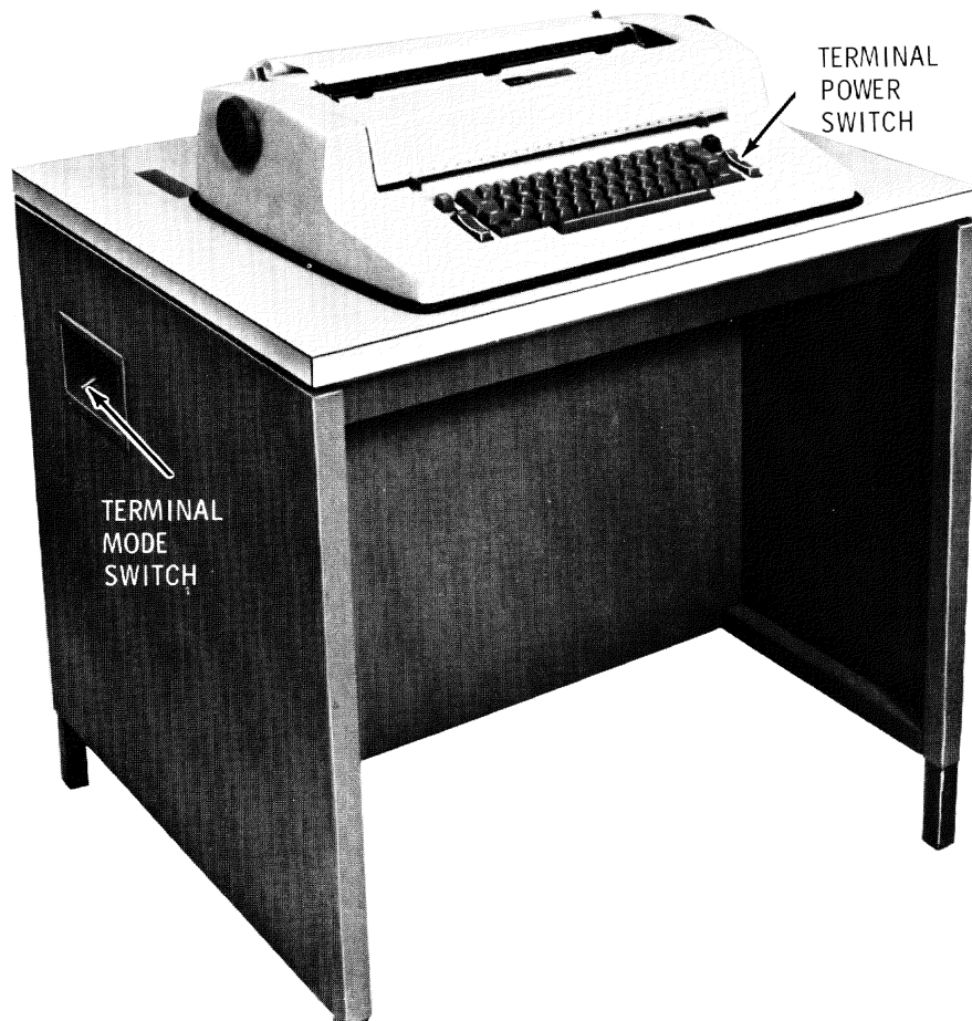
Figure A-4. 2741 Communications Terminal.
