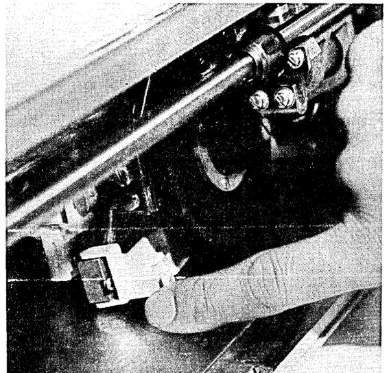
6. Turn the print wheel with your finger and make sure that the ink roll is rolling against the rear of the print wheel. If the ink roll is not rolling, remove the ink roll assembly and repeat this procedure starting from step 2.
