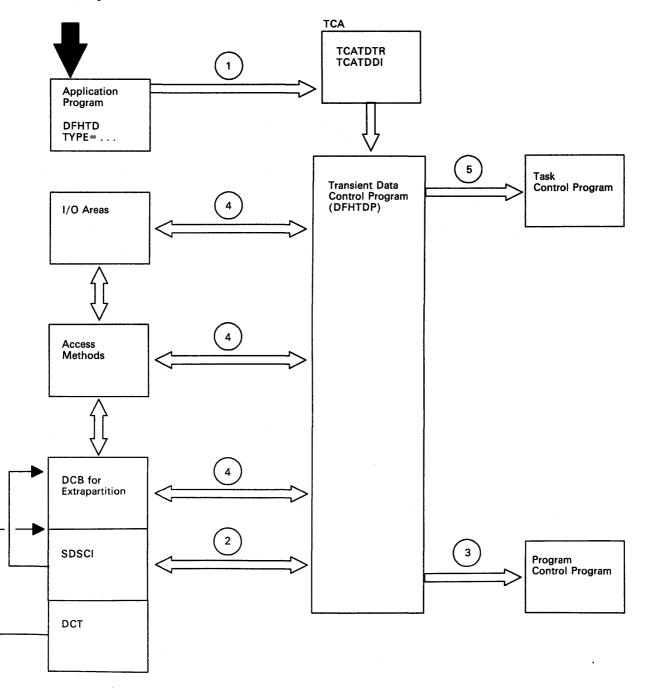
Figure 24. Transient Data Control Program Interfaces for Extrapartition
