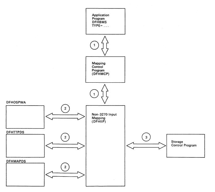
Figure 43. Non-3270 Input Mapping Interfaces
