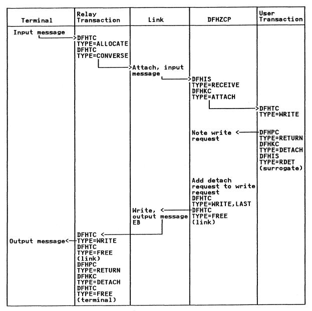
Figure 91. Flow for Message and Reply (No Wait)
