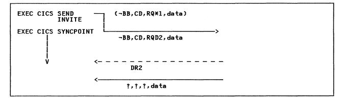
Figure 126. Two-Flow Sync Point with Deferred SEND INVITE
