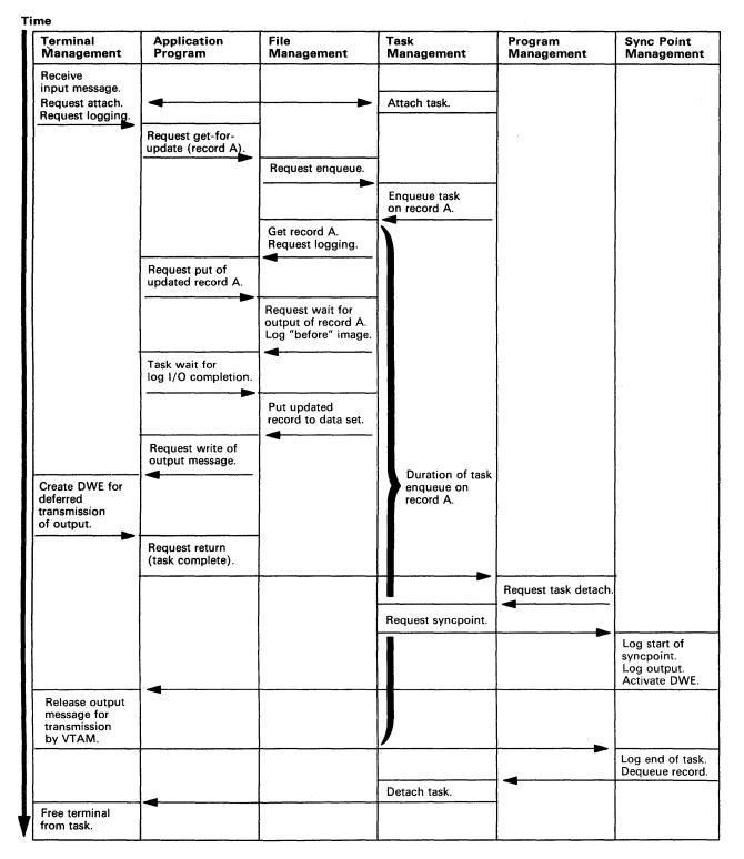
Figure 4. Flow of Control for a Simple Transaction (Including DWE Processing)
