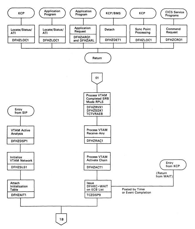
Figure 16 (Part 1 of 2). Terminal Management Common Control Routine
