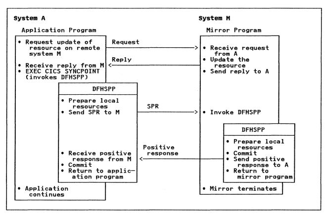
Figure 84. Sync Pointing with a Single Remote System
