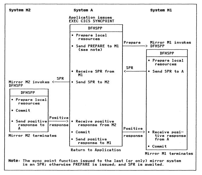
Figure 85. Sync Pointing with Multiple Remote Systems
