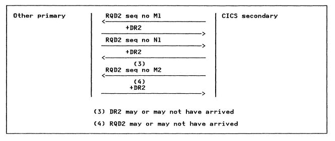
Figure 146. STSN Flows before First Type of Session Failure (CICS Secondary)
