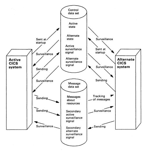
Figure 56. Use of the CAVM data sets for surveillance and tracking
