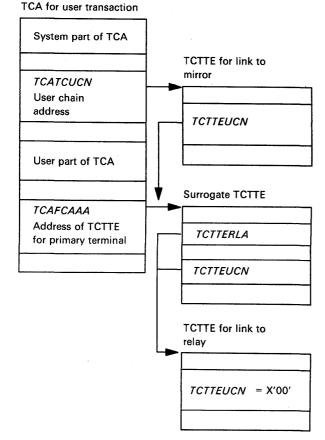
Figure 89. Control Blocks for User Transaction
