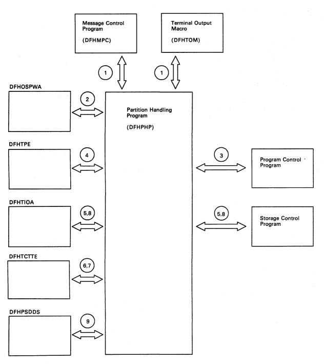
Figure 48. Partition Handling Program Interfaces
