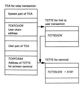
Figure 88. Control Blocks for Relay Transaction
