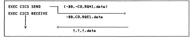
Figure 119. RECEIVE after Deferred SEND
