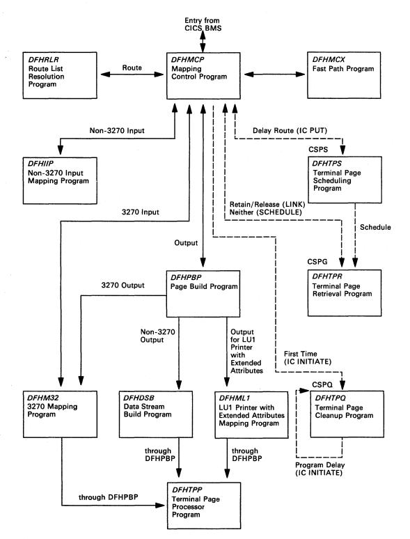
Figure 198. BMS Modules and Routines
