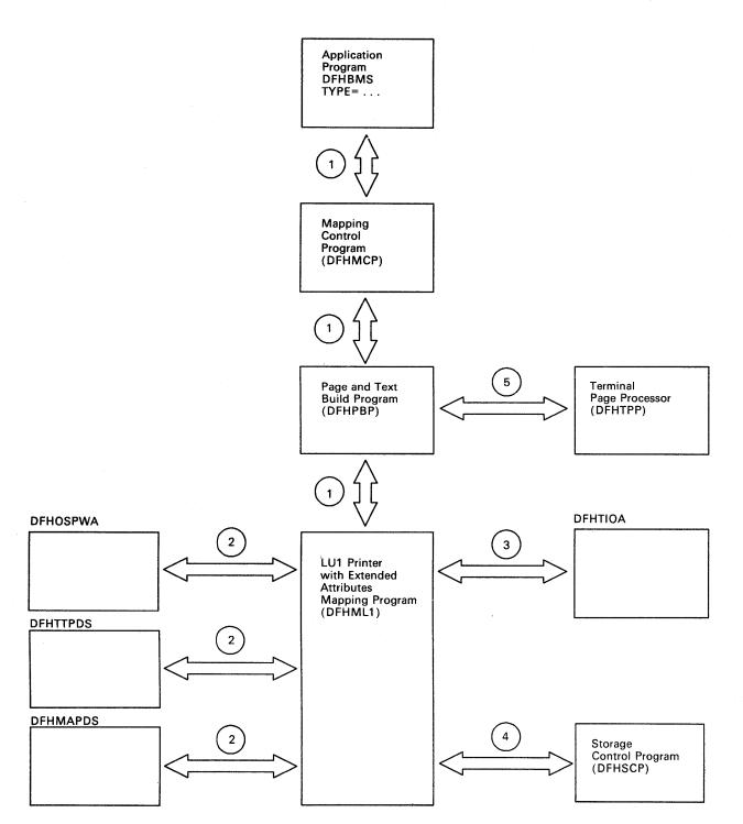
Figure 45. LU1 Printer with Extended Attributes Mapping Program Interfaces
