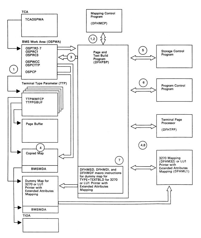
Figure 47. Page and Text Build Program Interfaces
