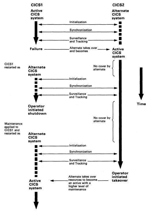
Figure 54. An XRF sequence
