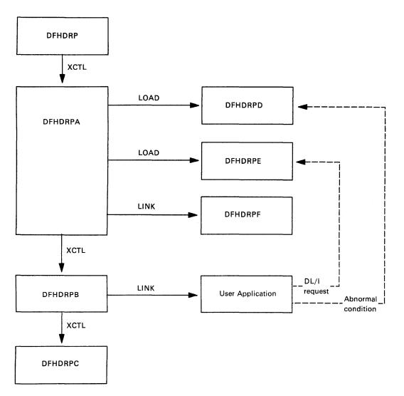
Figure 94. Interregion Communication - Batch Region Modules
