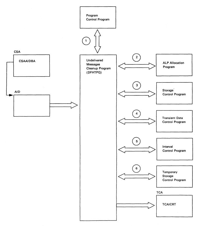
Figure 51. Undelivered Messages Cleanup Program Interfaces
