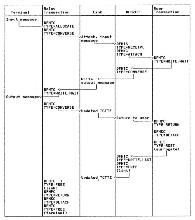
Figure 90. Flow for Message, Reply, and Wait
