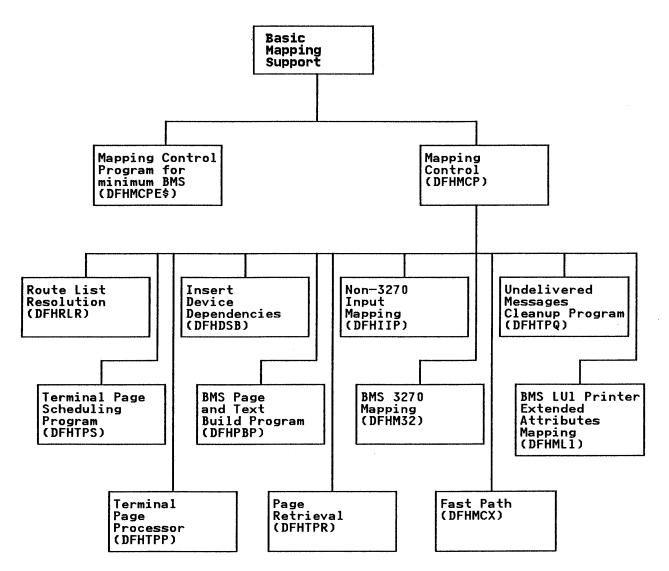
Figure 190. Basic Mapping Support
