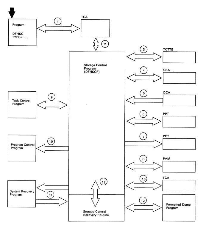
Figure 8. Storage Control Interfaces
