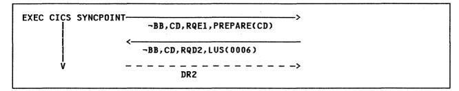
Figure 123. Three-Flow Sync Point without Deferred Data
