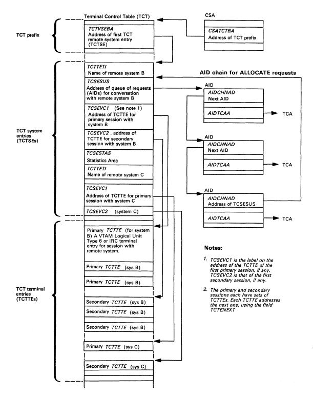
Figure 79. System Entries (TCTSEs) in Terminal Control Table
