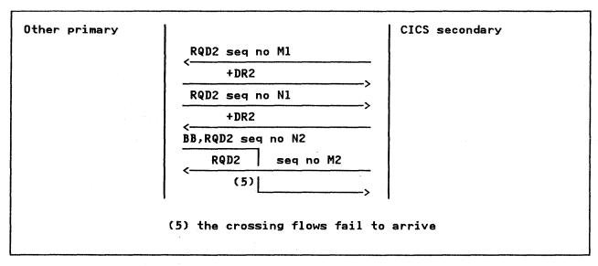
Figure 148. STSN Flows before Second Type of Session Failure (CICS Secondary)
