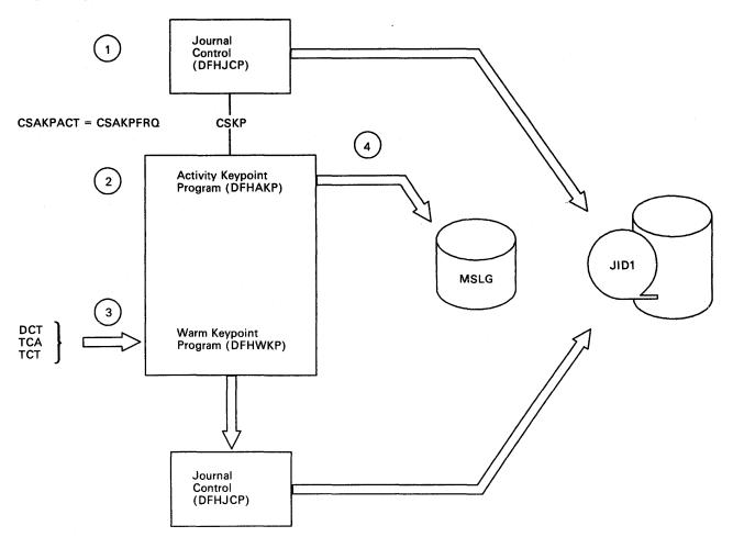
Figure 36. Keypoint Program Interfaces during Activity Keypointing
