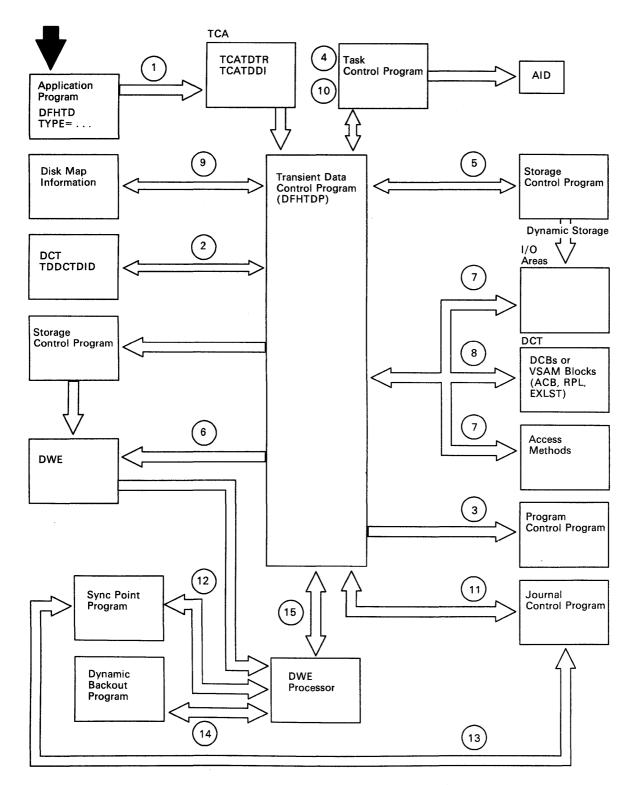
Figure 23. Transient Data Control Program Interfaces for Intrapartition
