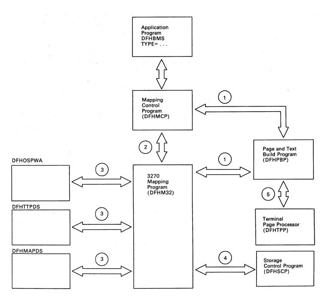
Figure 46. 3270 Mapping Program Interfaces
