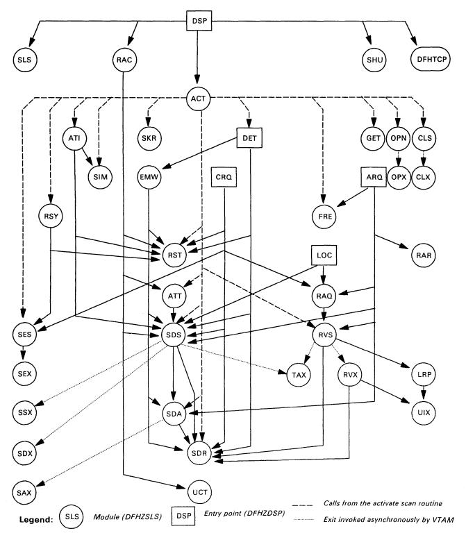
Figure 199. VTAM Terminal Management Control Flow
