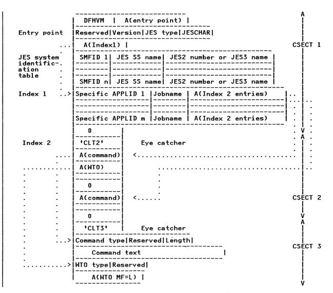
Figure 60. Structure of the CLT
