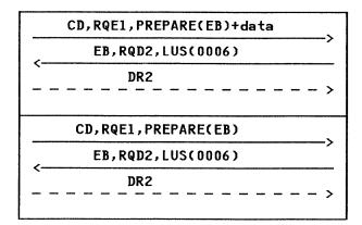
Figure 111. Three-Flow Sync Point, EB
