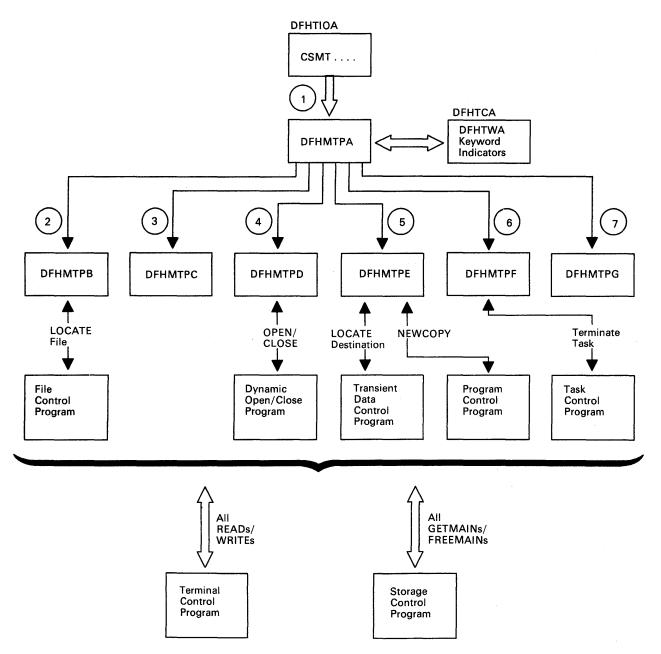
Figure 27. Master Terminal Program Interfaces
