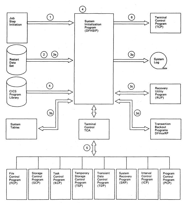
Figure 37 shows the relationships between the components of system initialization.
