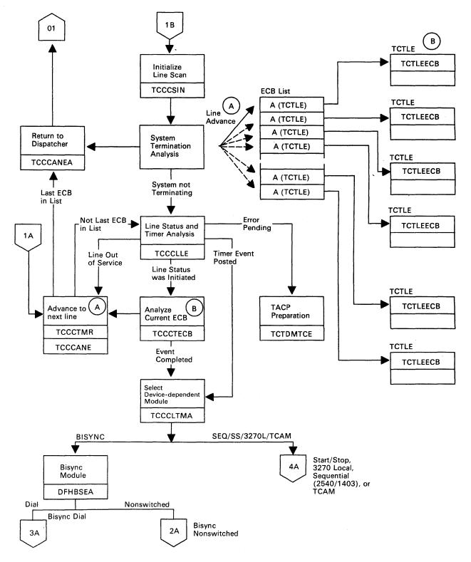
Figure 16 (Part 2 of 2). Terminal Management Common Control Routine
