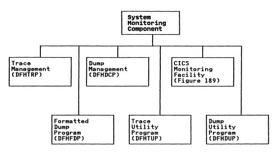
Figure 173. System Monitoring Component
