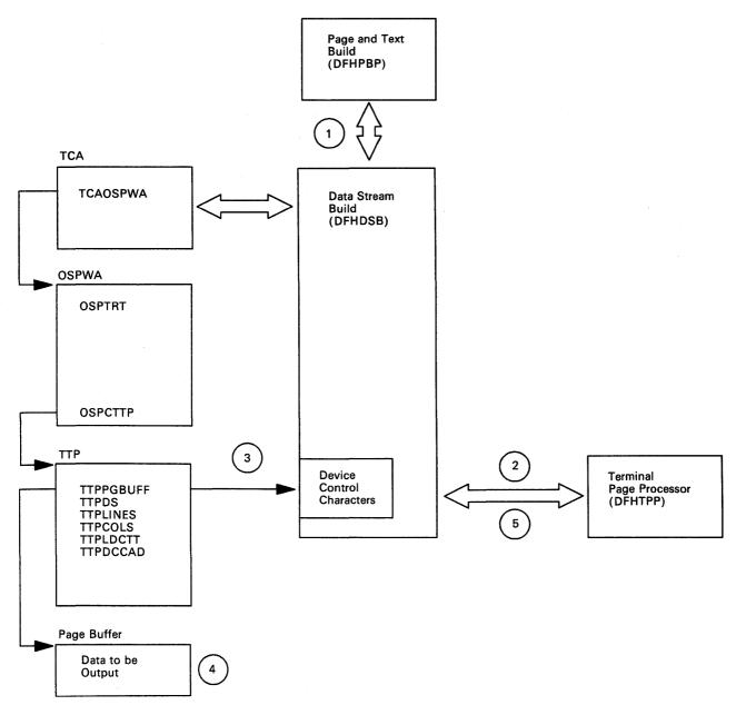
Figure 42. Data Stream Build Interfaces
