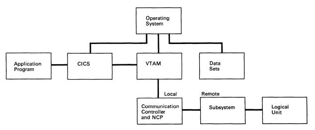
Figure 6. Interconnections between CICS System and an SNA Communications Subsystem
