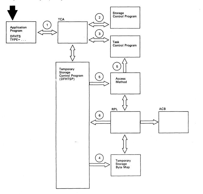
Figure 25. Temporary Storage Control Interfaces
