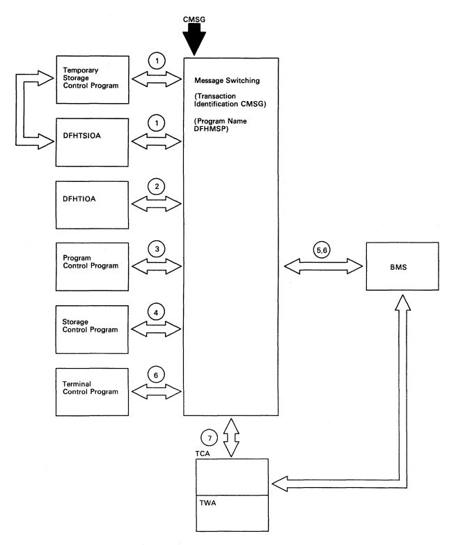
Figure 29. Message Switching Interfaces
