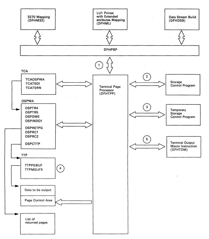
Figure 50. Terminal Page Processor Interfaces
