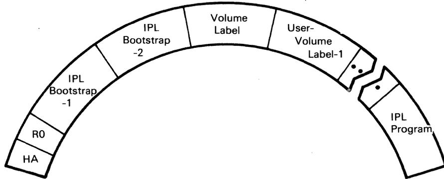
Figure 11. Cylinder 0, Track 0 Layout (Count Key Data Devices)
