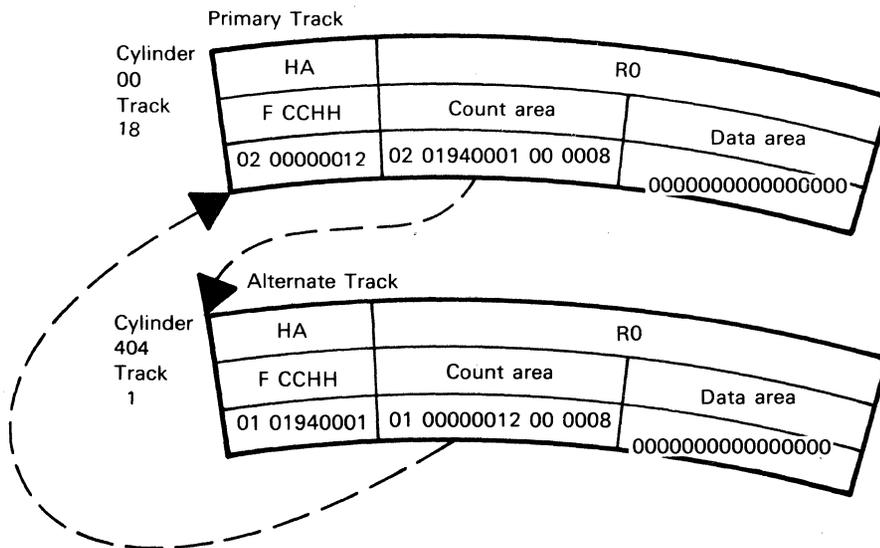
Figure 12. Primary/Alternate Track Association (Count Key Data Devices)
