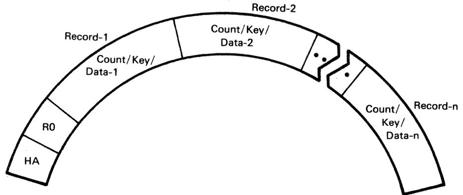
Figure 9. Standard Track Layout (Count Key Data Devices)
