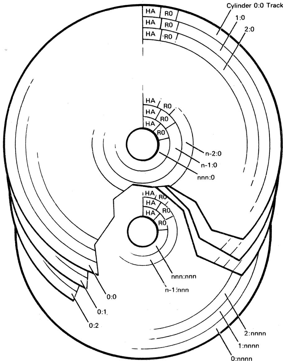
Figure 8. General Volume Layout (Count Key Data Devices)
