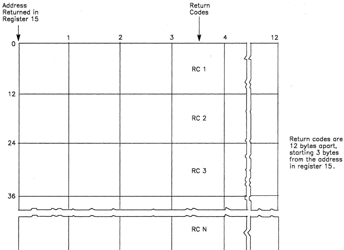
Figure 8. Return Code Area Used by DEQ
