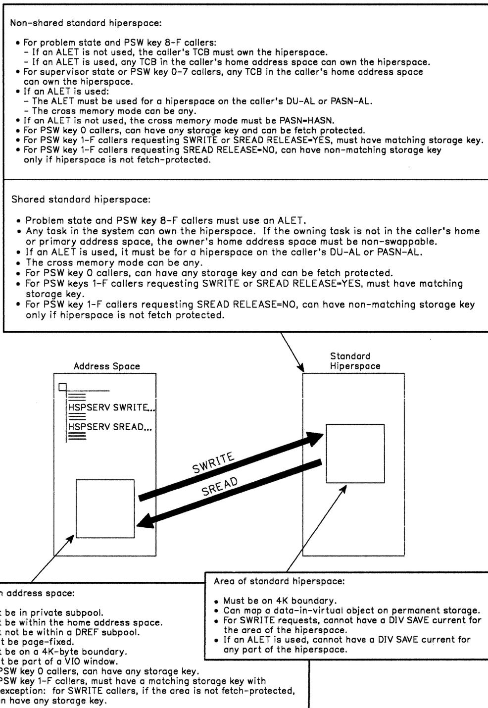
Figure 11. Characteristics and Restrictions for Standard Hiperspaces
