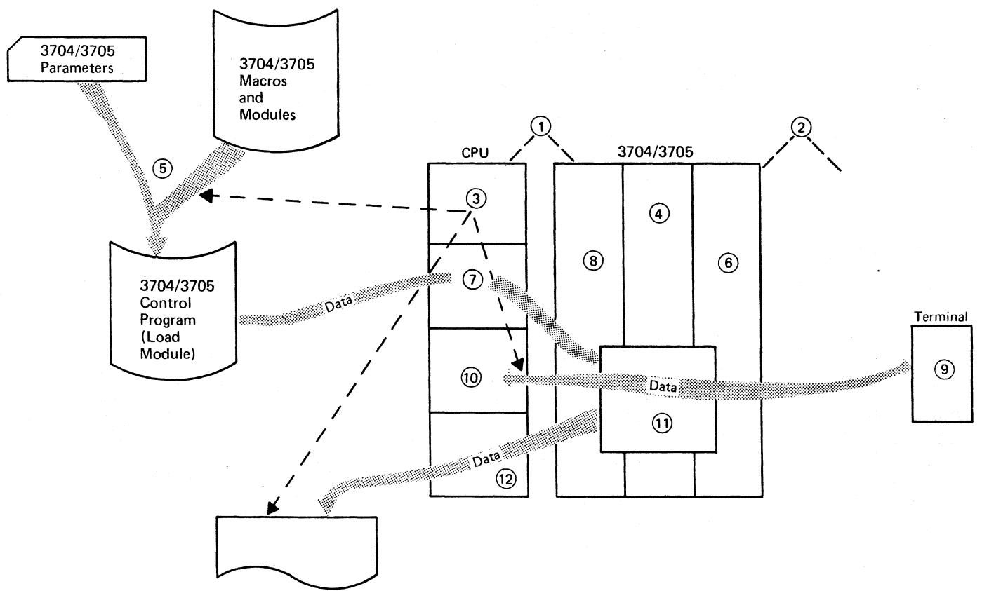
Figure 2 - 3704/3705 EP Component and Data Flow
