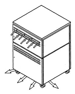
Figure 4-3. Direction of Airflow through a 3720 with a 3721
