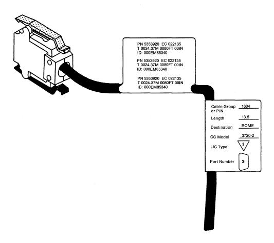
Figure 7-4. Label to be Attached to a LIC Cable
