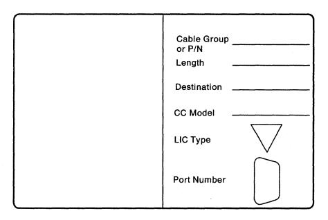
Figure 7-3. An Example of a LIC Cable Label
