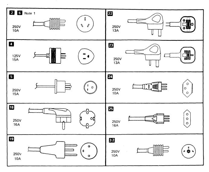
Figure 5-2. Power Plug Identification
