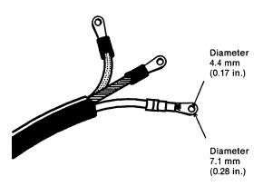
Figure 5-3. Power Cable Shipped without Plug
