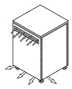
Figure 4-2. Direction of Airflow through a 3720
