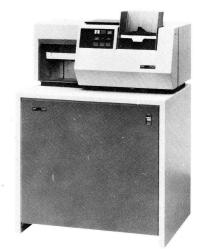
IBM 3782 Card Attachment Unit Model 2 with 2502 Card Reader (Attaches to 3774, 3775, 3776)
