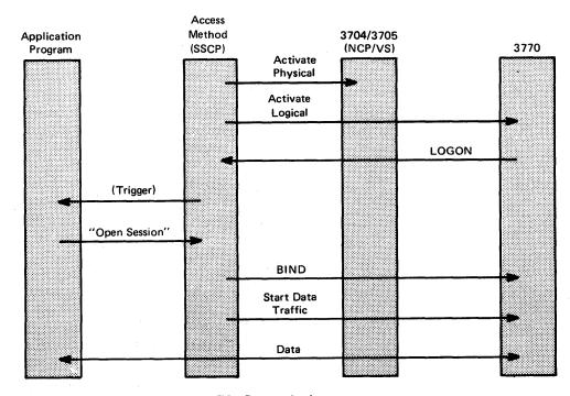
Figure 8-2. Example of Establishing SNA Communications
