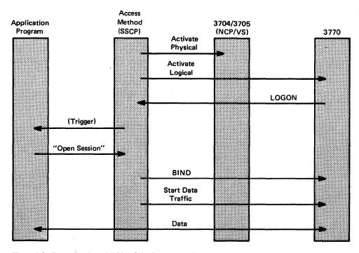
Figure 7-2. Example of Establishing SNA Communications
