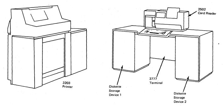
Figure 1-3. IBM 3777 Communication Terminal Model 1 Configuration
