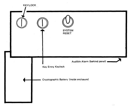
Figure 4-5. 3776/3777 MLU Auxiliary Operator's Panel and Battery Enclosure
