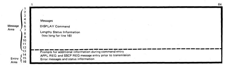
Figure 4-3 Console Display Areas and Uses
