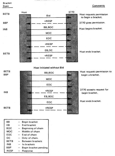
Figure 8-5. Examples of Bracket Protocol (2 of 2)
