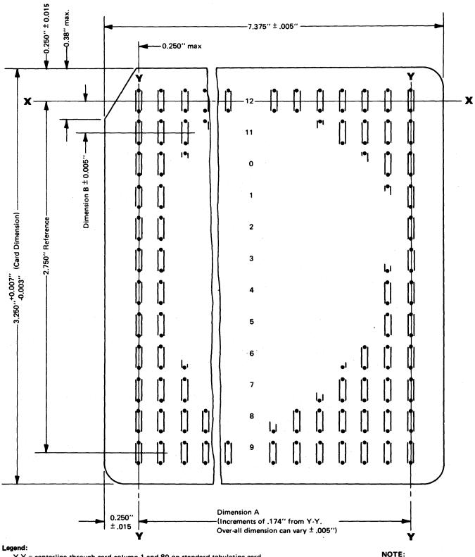
Y-Y = centerline through card column 1 and 80 on standard tabulating card.
