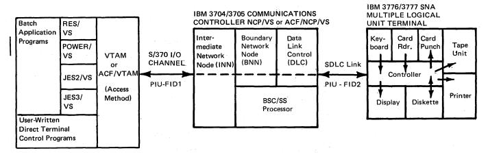
Figure 8-1. IBM 3776/3777 MLU Terminal in an SNA Network
