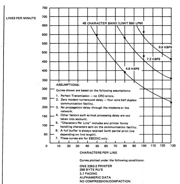
Figure D-10. One 3262-2 Printer, 48 Character Band-Nominal Throughput
