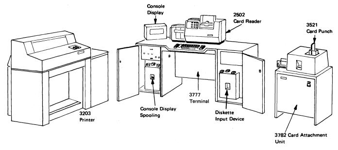
Figure 3-2. IBM 3777 Communication Terminal Model 2 Configuration
