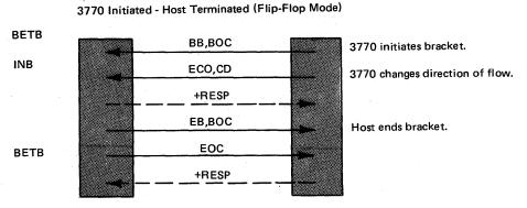
Figure 7-6. Examples of Bracket Protocol (1 of 2)
