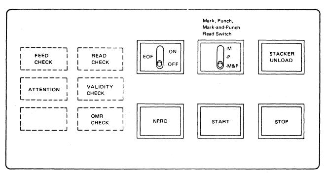
Figure 5-6. 2502 Operator's Panel
