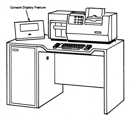
Figure 3-3. 3777 Model 2 Console Display Feature
