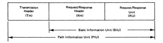
Request/Response Unit (RU): The basic unit of information in the data communication network. It may contain commands that control the flow of data through the network, responses to commands, acknowledgement of data, and optional data.
