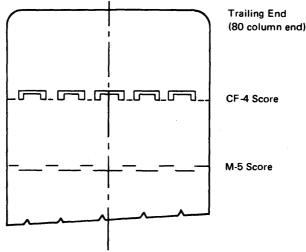
Figure C-1. Positioning of M-5 and CF-4 Scores
