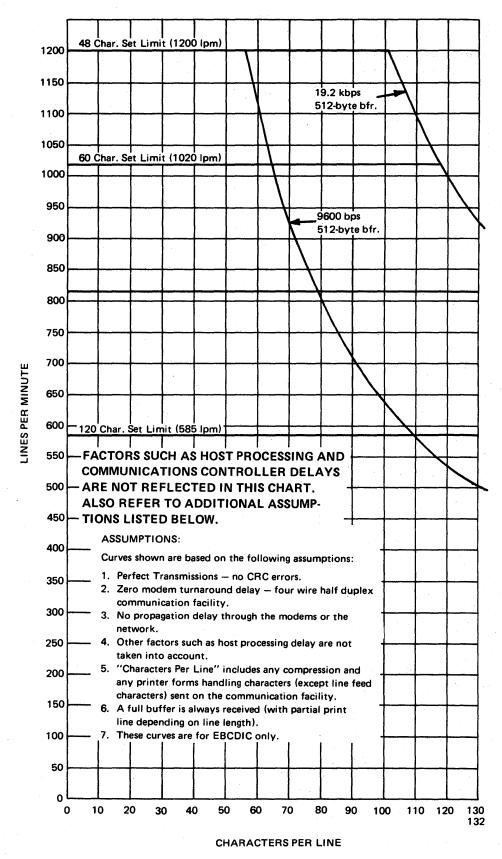
Figure D-9. 3777 Model 1 Line-to-Printer (1200 lpm) Throughput (SDLC)
