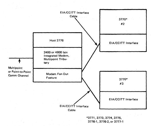
Figure 2-5. Modem Fan Out Configuration
