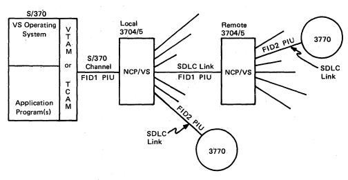
Figure 7-1. Example of an SNA Network
