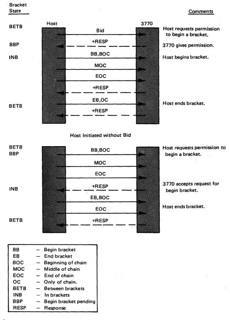
Figure 7-6. Examples of Bracket Protocol (2 of 2)
