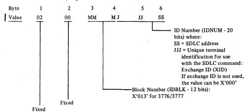
For example, assume a 3776 terminal with JJJ = X'00B' and SS = X'C1'. The terminal ID bytes from the 3776 would be sent to the CPU as:
