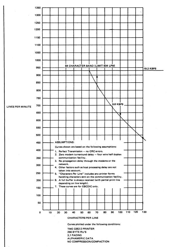
Figure D-13. Two 3262-2 Printers, 64 Character Band-Nominal Throughput
