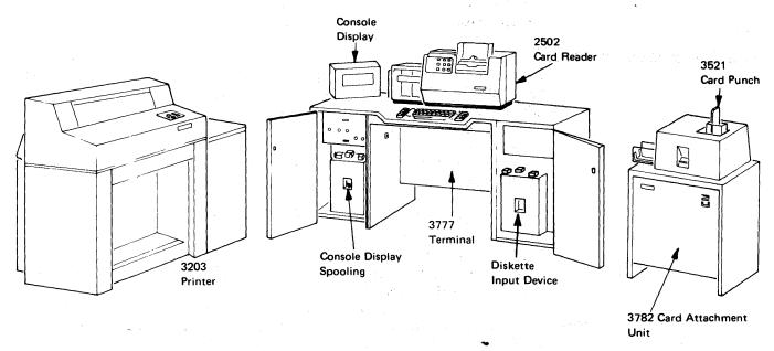
Figure 1-5. IBM 3777 Communication Terminal Model 2 Configuration
