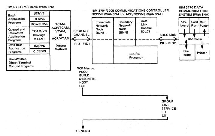
Figure 7-8. IBM 3770 Communication Terminal in an SNA/SDLC Network
