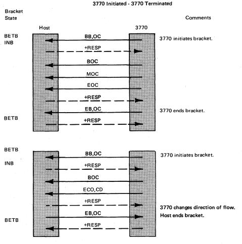
Figure 8-5. Examples of Bracket Protocol (1 of 2)
