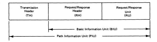
Request/Response Unit (RU): The basic unit of information in the data communication network. It may contain commands that control the flow of data through the network, responses to commands, acknowledgement of data, and optional data.
