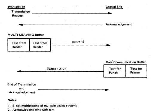
Figure 3-1. Example of How MULTI-LEAVING Works
