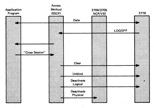
Figure 8-3. Example of Terminating SNA Communications
