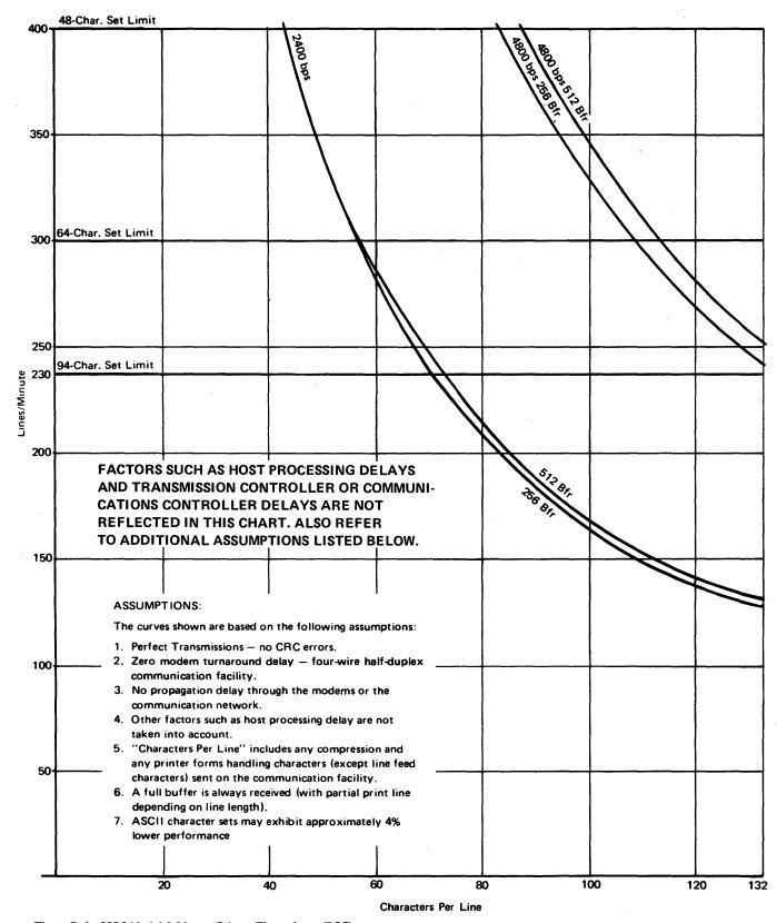
Figure D-4. 3776 Model 2 Line-to-Printer Throughput (BSC)
