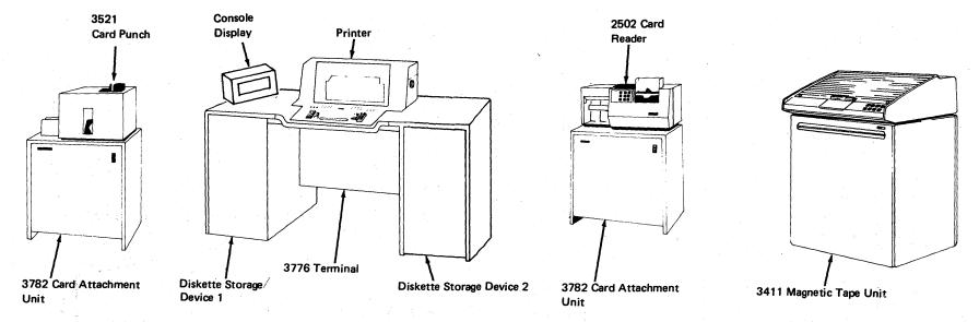
Figure 1-6. IBM 3776 Communication Terminal Model 3 or 4 Configuration
