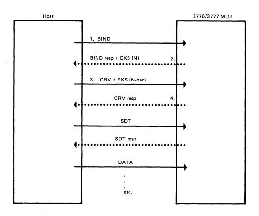
Figure 4-4. Example of Establishing a Cryptographic Session
