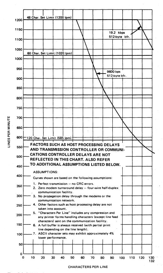
Figure D-8. 3777 Model 1 Line-to-Printer (1200 lpm) Throughput (BSC)
