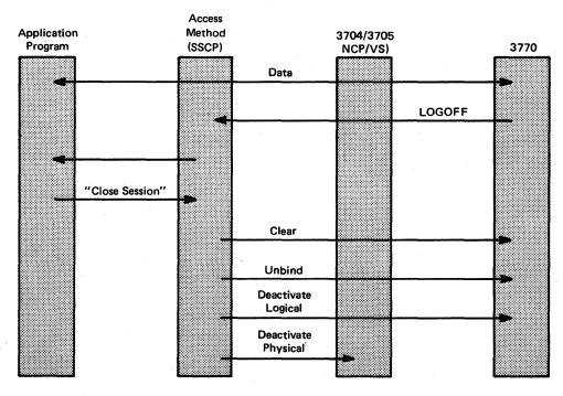
Figure 7-3. Example of Terminating SNA Communications
