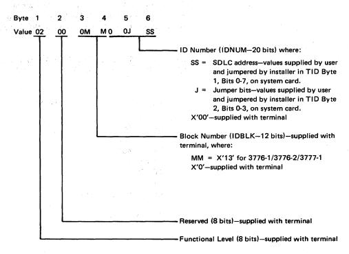
For example, assume a 3776 terminal with J = X'B' and SS = X'C1'. The terminal ID bytes from the 3776 would be sent to the CPU as:
