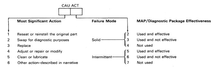
**Note:** Consider the MAPs and diagnostics effective if they identify the failing part or direct you to the appropriate repair action or procedure.
