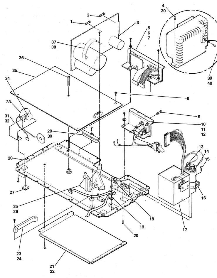
FIGURE 3. BASE PLATE ASSEMBLY. SEE LIST 3.
