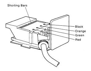
Figure 16-9. IBM Cabling System Data Connector (Interior View)
