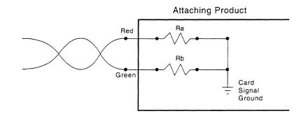
Figure 16-7. Resistances Seen from Phantom Drive
