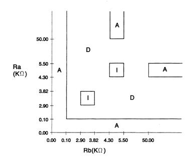
Figure 16-8. Active and Inactive Wire Fault Regions
