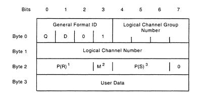
Figure 3-4. Data Packet Format in Modulo 8
