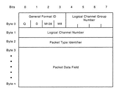
Figure 3-3 shows the general structure of an X.25 packet.
