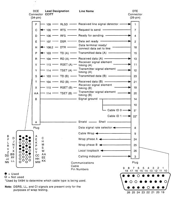
Figure 16-5. V.35 Interface Lines between the DTE and DCE
