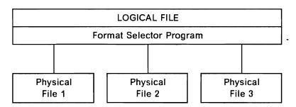
Figure 14. Format Selection - Diagram of Logical File and Three Physical Files
