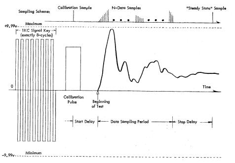
Figure 4. Format of input signal to the analog-to-digital subsystem.
