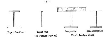
For purposes of computation the flange plates are assumed to be 16 inches wide. If the negative moment exceeds the positive moment no composite design is made.
